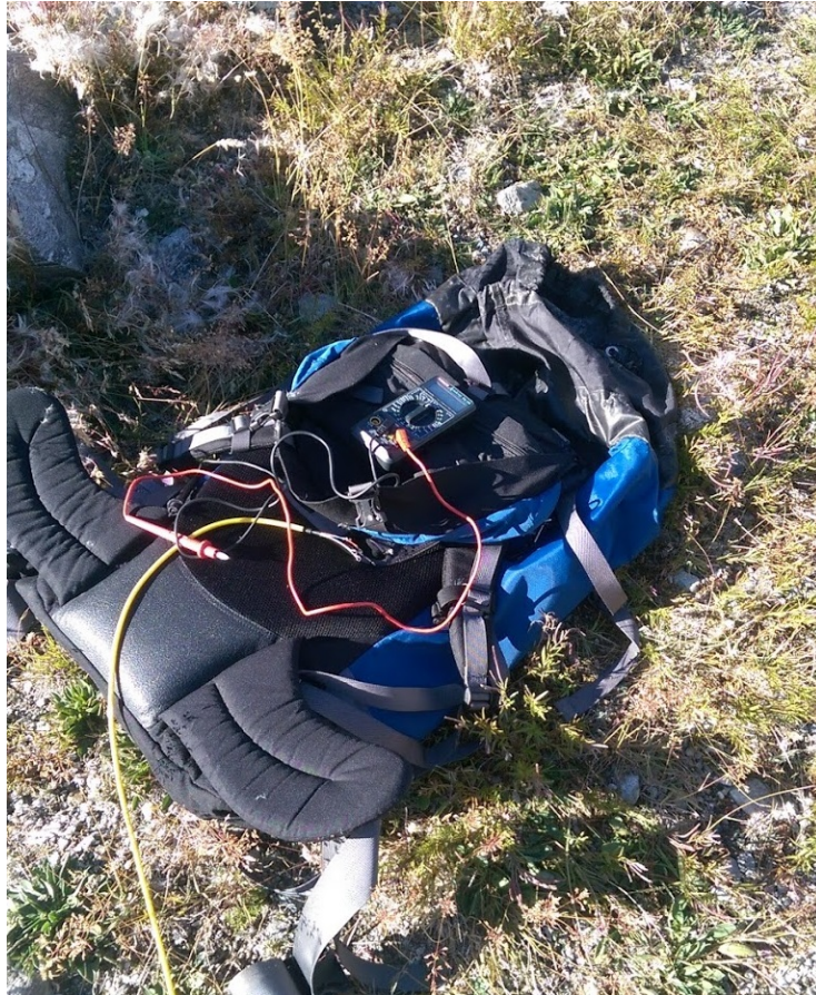
Figure 4.3: Kipp and Zonen CMA6 Albedometer wired to multimeter taking voltage readings.
