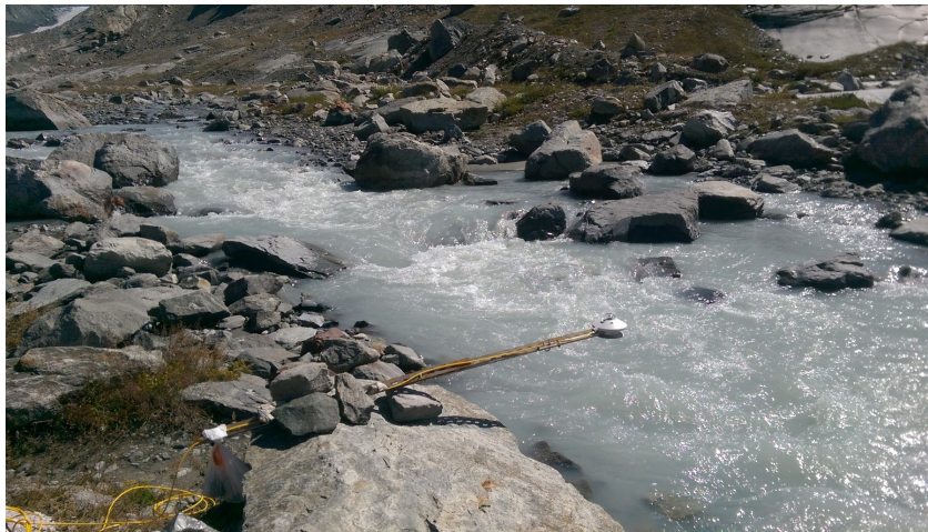
Figure 4.1: Kipp and Zonen CMA6 Albedometer in position 1.5 m above the surface of the Findelenbach study site, close to the Findelenbach gauging station ( 46.00^\circ , 7.81^\circ ).
