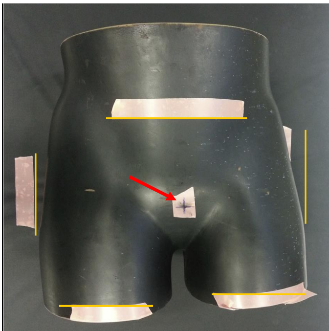
Figure 17 - anthropomorphic pelvis phantom used for the study, which is marked with a centring point (red arrow) and collimation borders (yellow lines)
