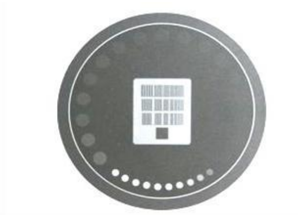
Figure 12 – TOR CDR Leeds Test Object used in radiography (Leeds Test Object Ltd, North Yorkshire, United Kingdom).
