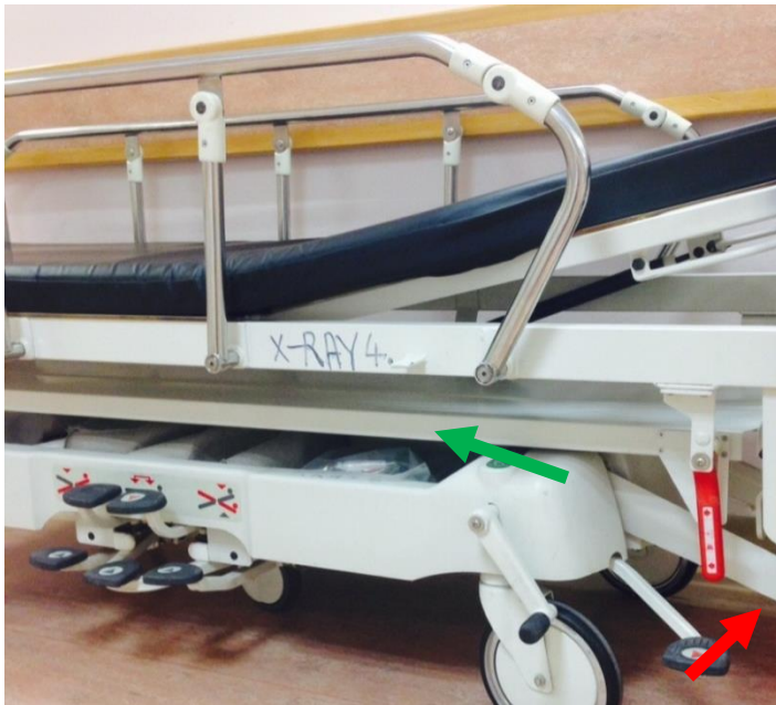
Figure 3 – Trolley with PLATFORM (green arrow) underneath it which can be elevated with the red handle (red arrow) (Lifeguard 50 trolley, ArjoHuntleighs' Healthcare, Sweden)
