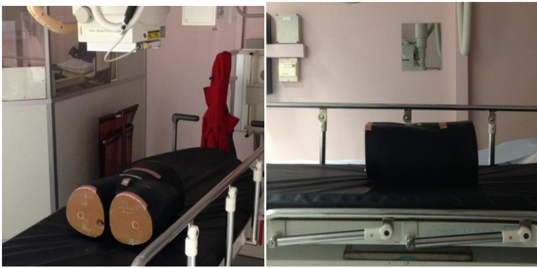
Figure 19 - images demonstrating the positioning of the phantom for an AP pelvis on the trolley with the image receptor placed on the platform below.
