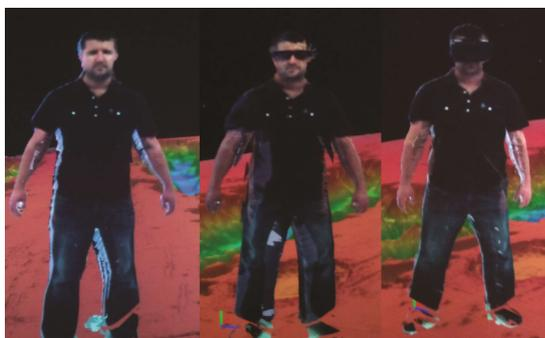
Fig. 9. This figure demonstrates the occlusion problem for the viewer when using various display devices. Left no stereo (full facial expressions), center stereo glasses (eye gaze and some facial features obscured) and right HMD (Most of the face obscured. identification of facial expressions not possible).
