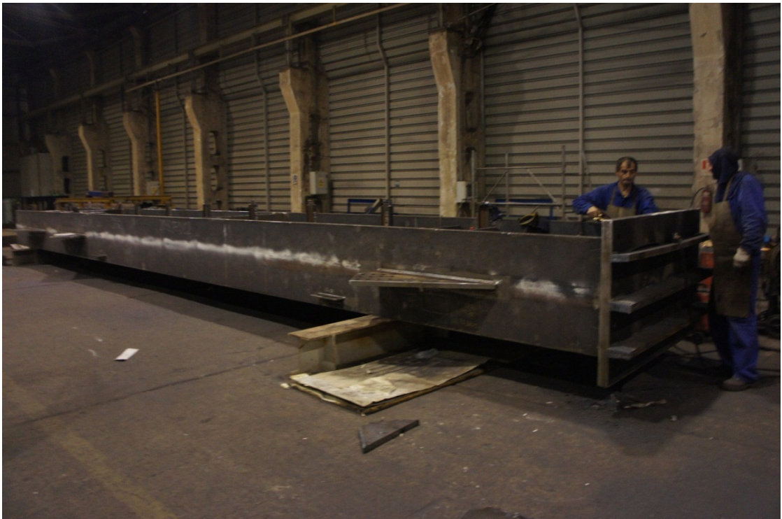
Photograph 46: 2014-09-04 – Romania factory with column elements under fabrication
