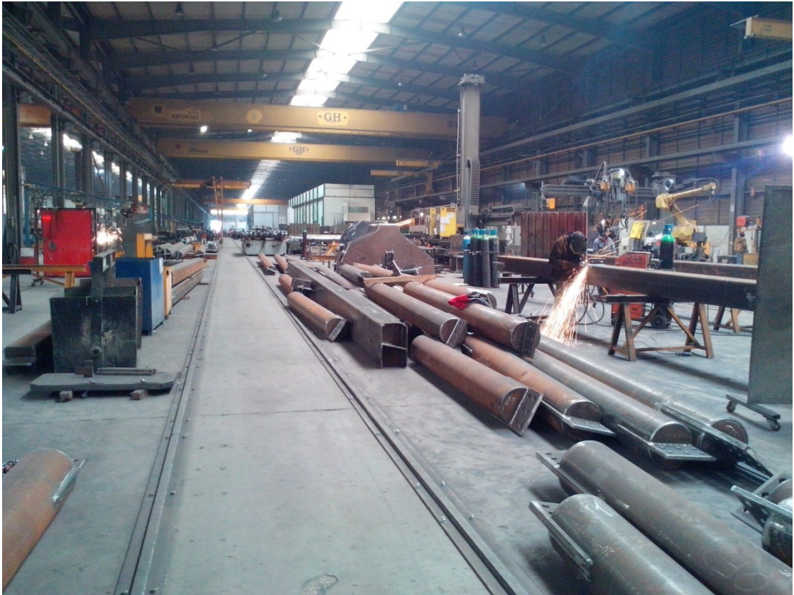
Photograph 45: 2014-09-11 – Portugal factory with beam-bracing elements under fabrication
