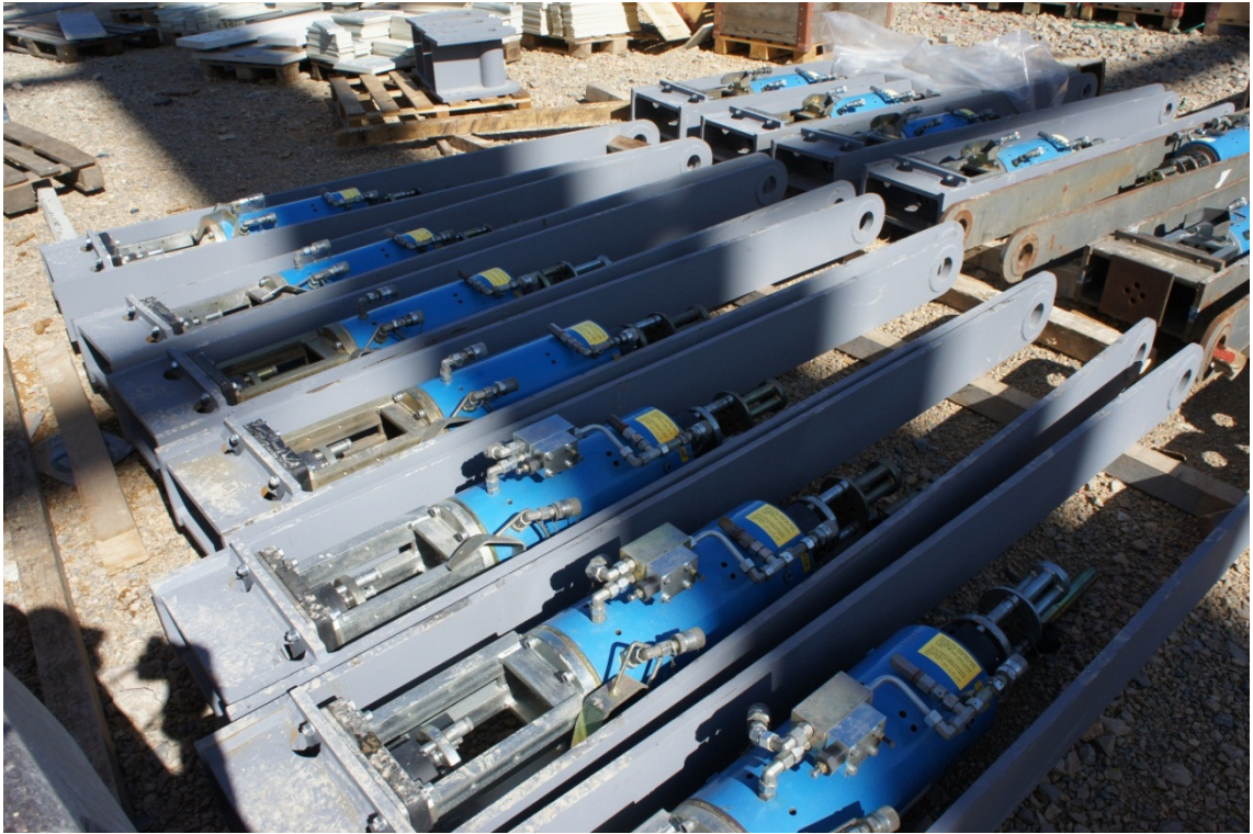
Photograph 13: 2015-08-25 – synchronised lifting jacks ready for installation
