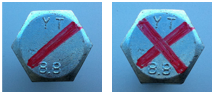
Figure 9.31: Bolt annotation after the first and second tightening steps (by Subcontractor)
