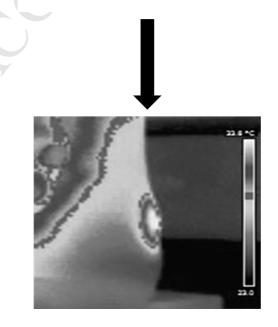
Hot spot development measured using infrared thermography
