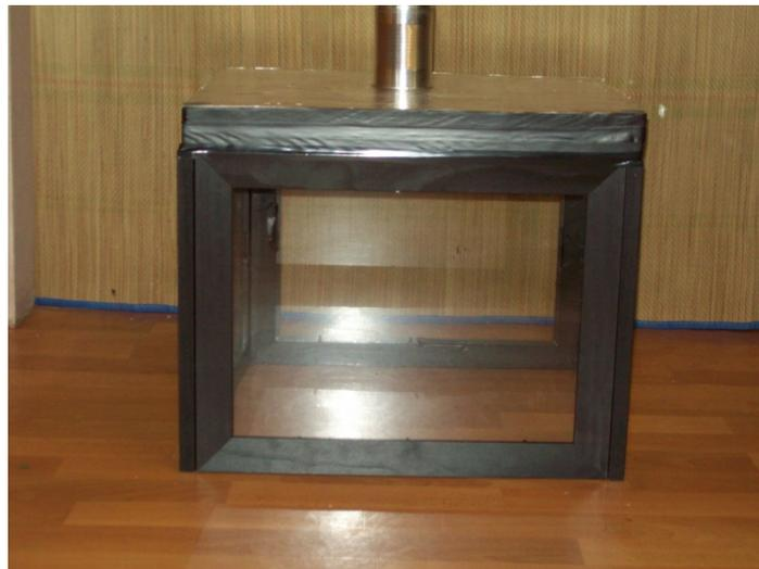
[Figure 6.5: Ignitability Test Cabinet](#)
