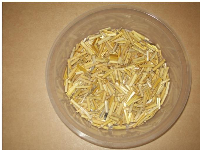
Figure 3.26: Straw Cut to 10mm – 15mm
