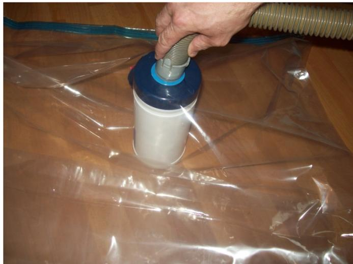
[Figure 3.36: Photo Showing Air Being Sucked out of Vacuum Bag](#)
