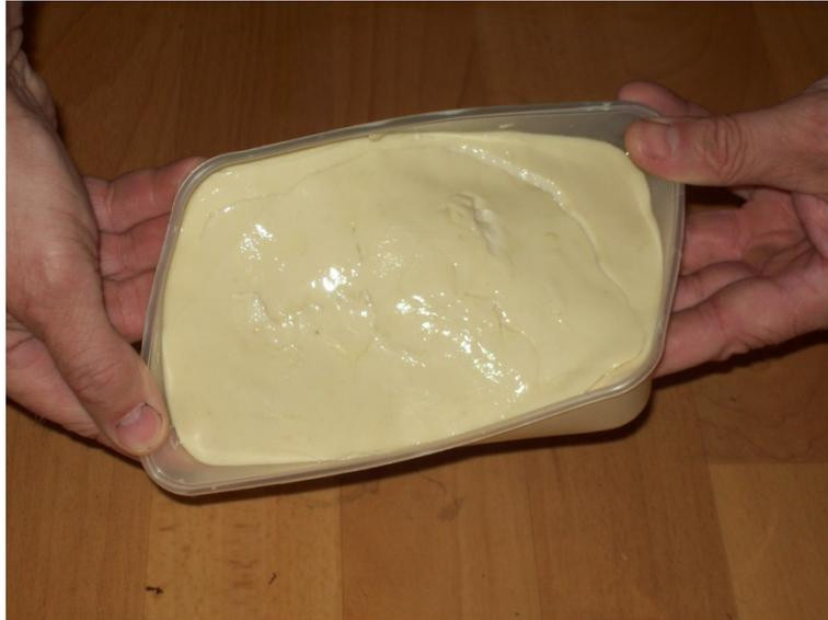
[Figure 3.22: Waste Engine Oil Set to a “Blancmange” State](#)
