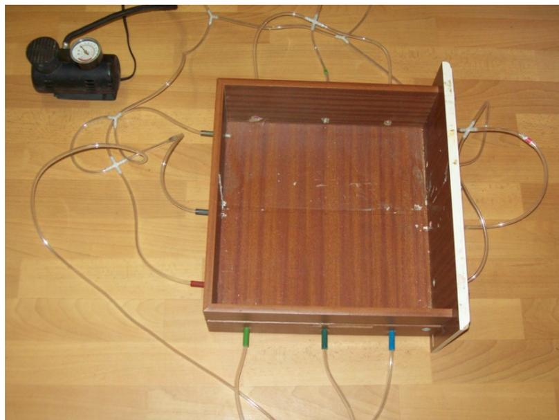
Figure 3.35: Aerating Box with Air tubes and 12v Compressor
