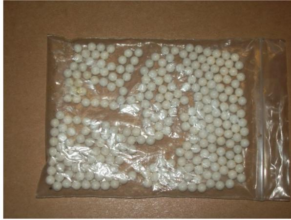
[Figure 3.29: 10mm PEHD Hollow Spheres](#)
