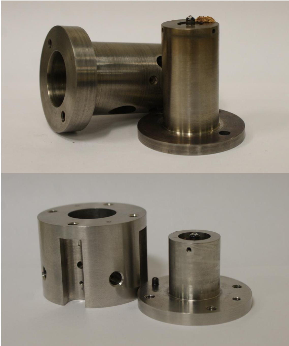
Figure 4.2: Photographs of custom-made diamond anvil cells. (top) HT2, based on a Mao-Bell type piston-cylinder cell for use in combination with resistive heaters in experiments at combined high pressure and temperature. (bottom) TE3, a piston-cylinder cell suitable for experiments at ambient temperature.
