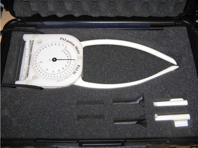
Figure 7. Palpation Meter (PALM) (Performance Attainment Associate, St. Paul, MN, USA)
