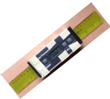
Figure 15. The inclinometer was adapted with a 30cm plastic ruler attached along the length of the inclinometer, and the ruler was used to align the inclinometer between the Olecranon Process to the Ulnar Styloid.
