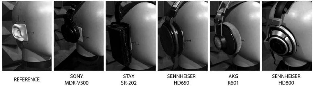
Fig. 1. Headphone sets mounted on B&K HATS for physical measurement stage of the investigation.
