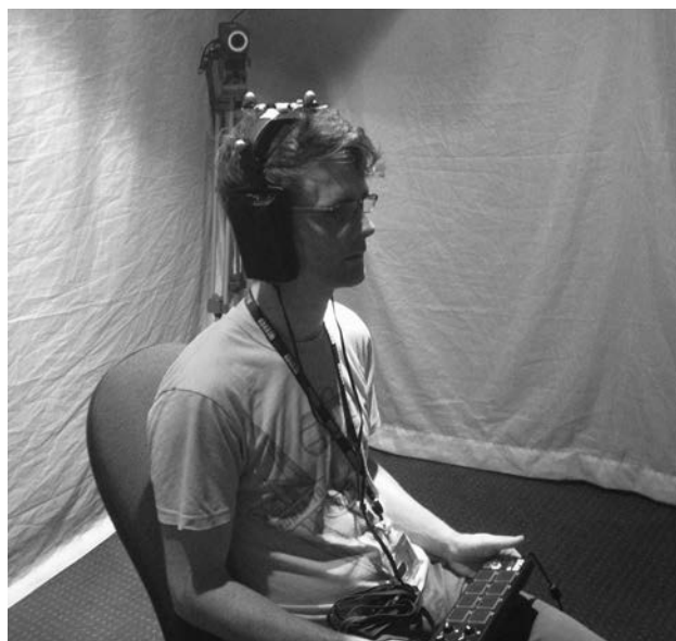
Fig. 6. A picture demonstrating how listeners participated in the test. The response device can be seen on the participants lap. Reflective markers are visible mounted to the top of the headphones and one of the four tracking cameras can be seen in the background.
