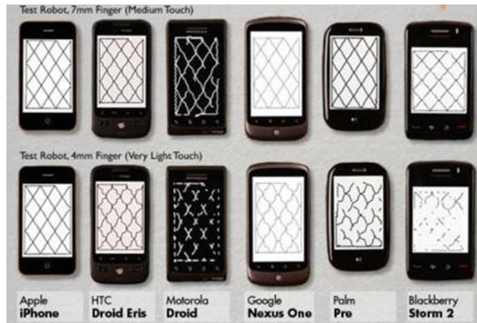
Figure 2.1: Tracing Tests on Different Devices
