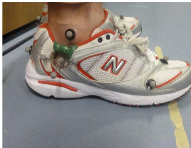
Figure 3.2. Triad marker. This marker was attached to the heel through the heel counter of the shoe.
