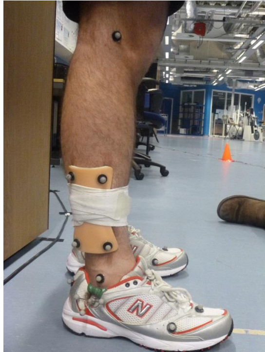
Figure 3.3. Marker placement. The figure illustrates the marker placement for heel and leg technical markers, and femoral, malleoli and foot anatomical markers viewed from the sagittal plane.
