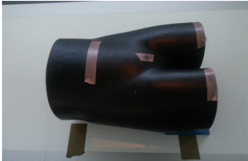
Figure 6-1. Anthropomorphic pelvis phantom used in the current study.
