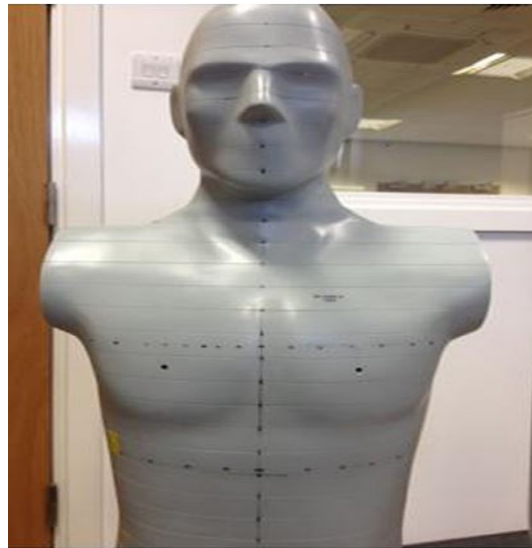
Figure 6-2. A CIRS ATOM adult phantom for direct organs' doses measurement using TLD.
