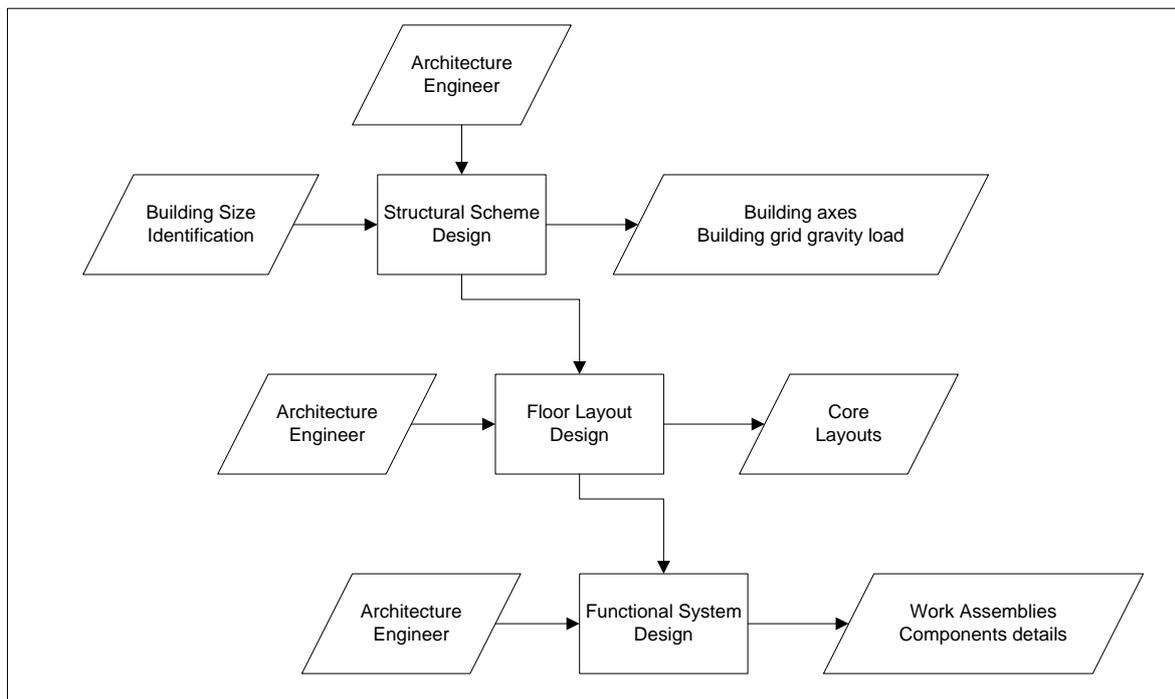
Figure 2-1 the sub-stages of structural engineering design (Sacks et al., 2000)
