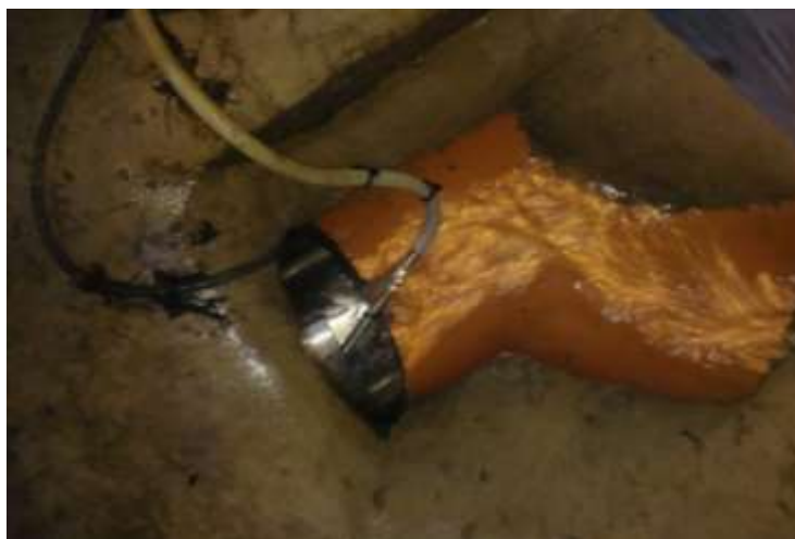
Figure 20 - (left) View up the pipe showing the placing of the flow sensor Figure 21 - (above) View showing fixing of the sample line in the chamber
