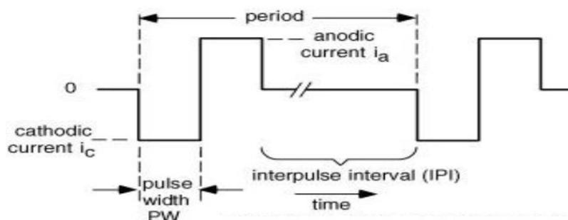
**Figure 2.7: Typical waveform for FES (Merrill et al., 2005). The narrow pulse width is indicated PW. The interpulse interval (IPI) is the time between pulses.**
