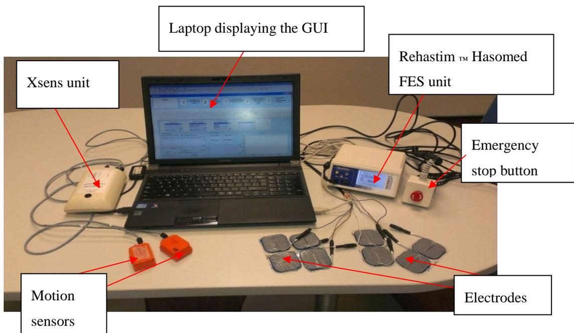
**Figure 7.1: The final prototype UL FES Rehab Tool – software and hardware components**
