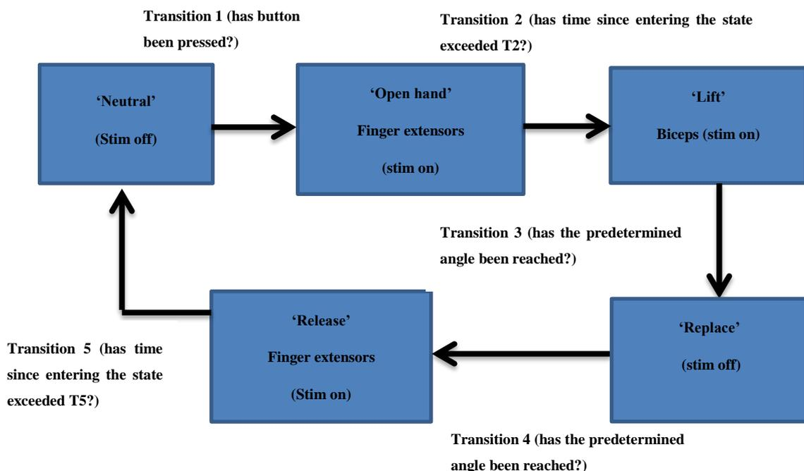
Figure 3.3: Example FSM for drinking from a glass. Boxes represent the states and T1-T5 the transitions between states.
