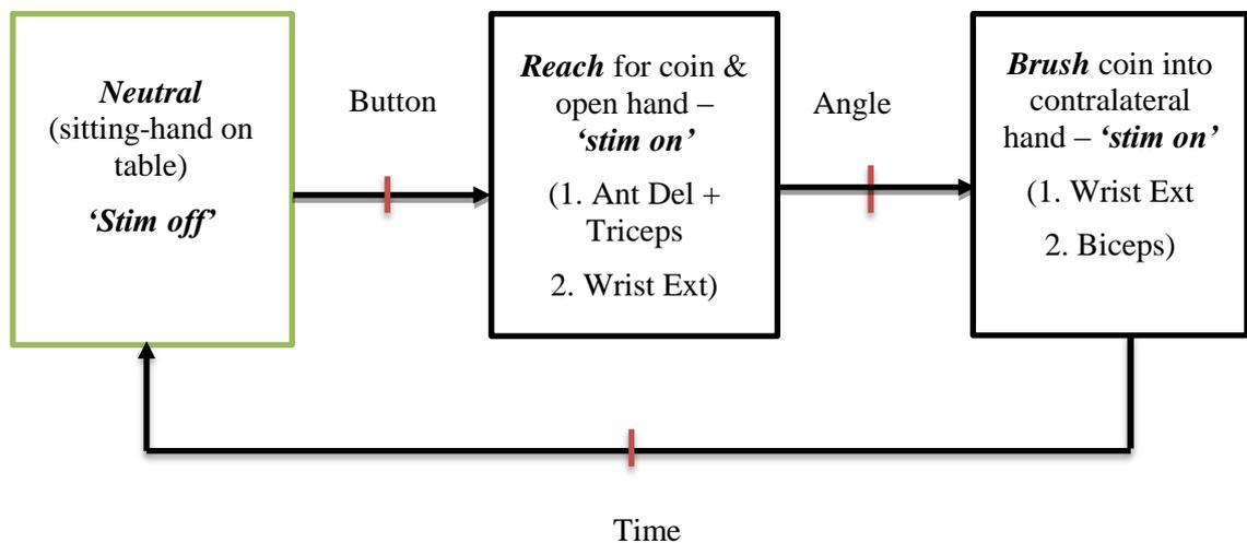
**Figure 5.8: State machine diagram for sweeping coins into contralateral hand.**
