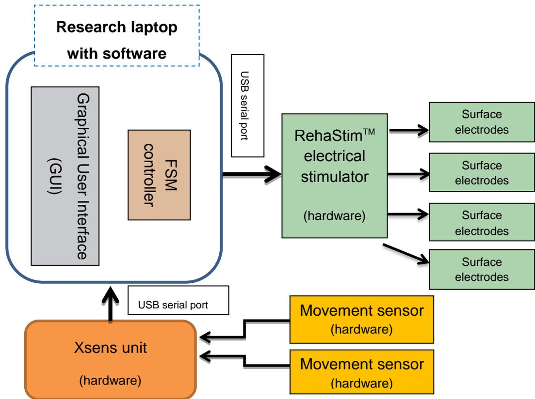
**Figure 3.4:** Graphical representation of the laptop with GUI, RehaStim™ (FES unit) and surface electrodes, the inertial sensor system (Xsens) with 2 inertial measurement units (each comprising a 3 axis accelerometer, 3 axis gyroscope and 3 axis magnetometer).
