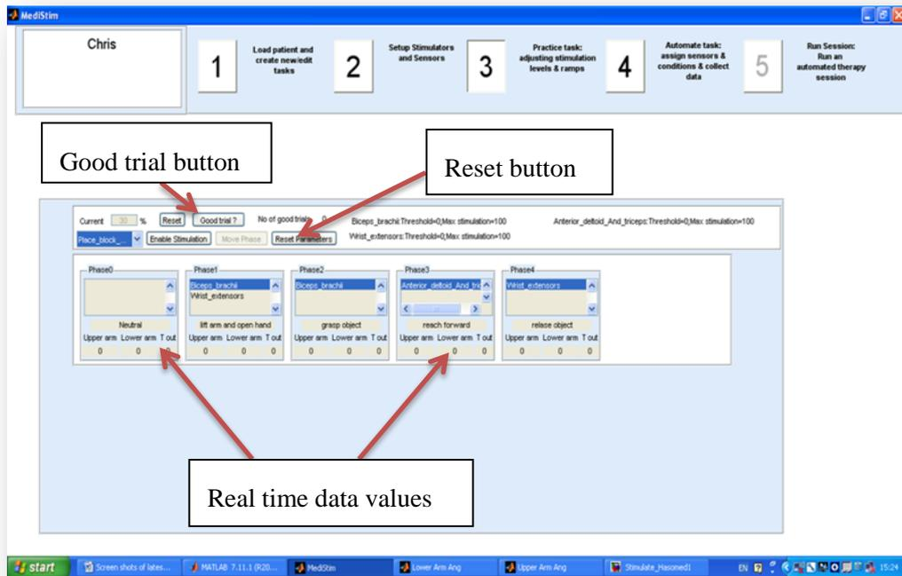
**Figure 5.10:** Screen shot of stage 3 GUI , v3.0 following changes. Note addition of good trial, rest buttons and windows showing real time data capture for angles and time elapsed.
