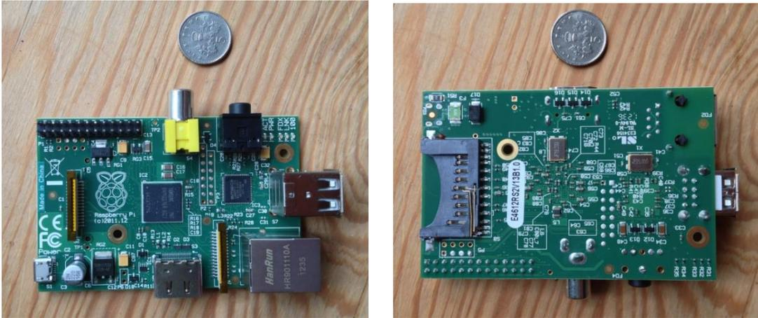
**Figure 3.7 Top (left) and underside (right) of the Raspberry Pi (RPi) computer, with a UK 5 pence coin for scale**
