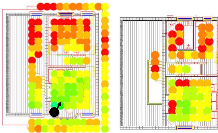
**Figure 5.2. Spectrum analyzer results from Test 2 at the Salford Energy House, ground floor (left) and first floor (right)**
