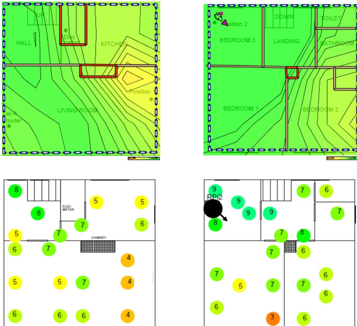
**Figure 6.2 The simulated signal contour map (above) and actual signal strength results (bottom) from triple point position 2 at Home1, ground floor (left) first floor (right)**
