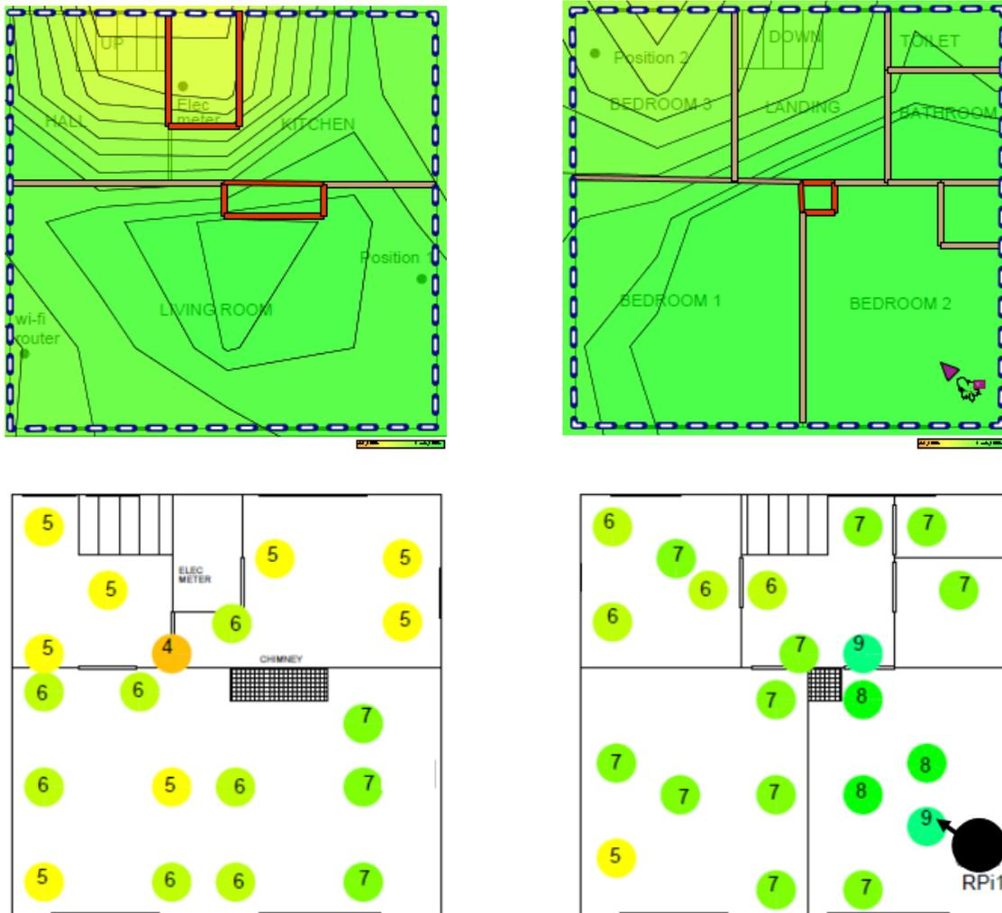
**Figure 6.1 The simulated signal contour map (above) and actual signal strength results (bottom) from triple point position 1 at Home1, ground floor (left) first floor (right)**
