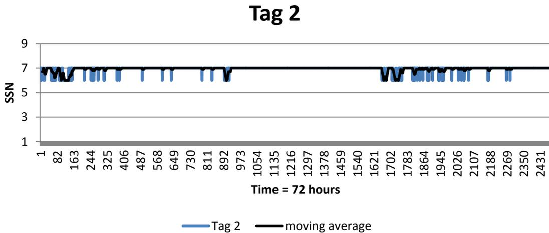
**Figure 5.49 Tag 2 signal strength over 72 hours in the Environmental Effects Test 3**
