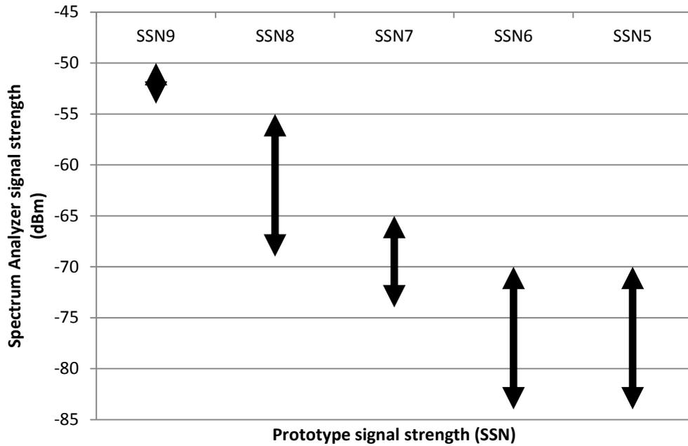
Figure 5.19. Comparison of spectrum analyzer and prototype signal strength
