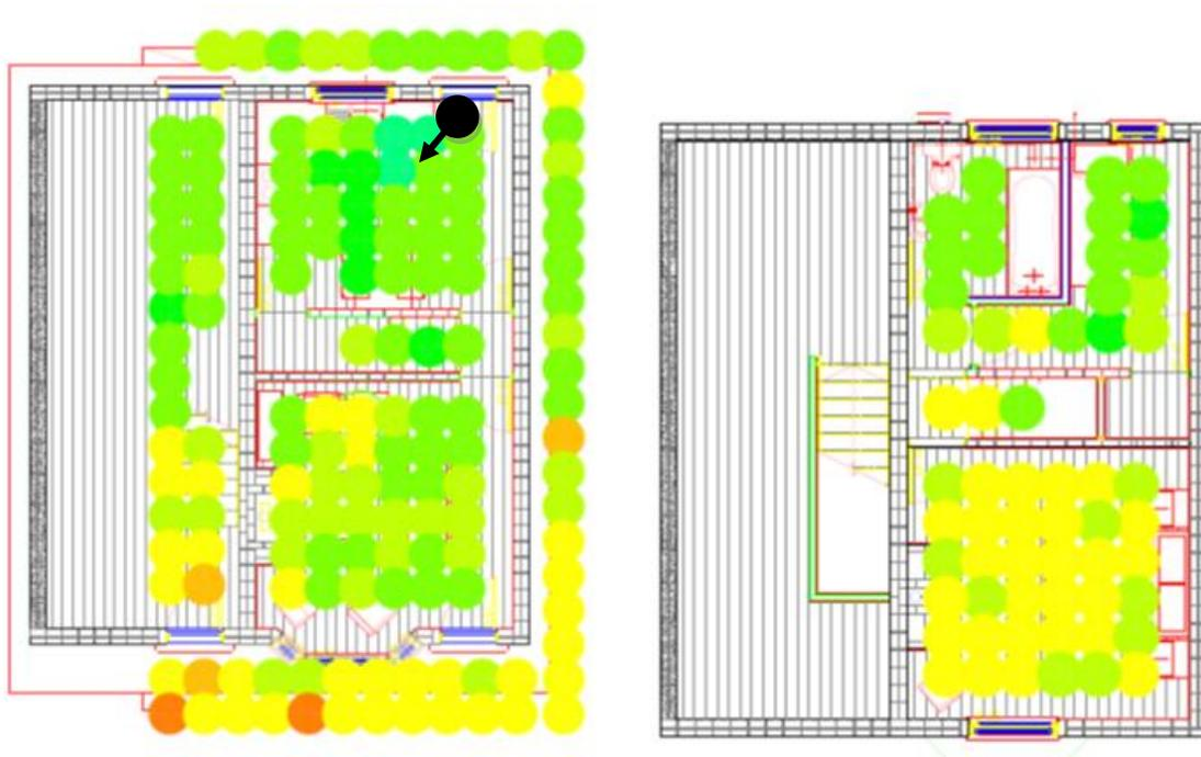
**Figure 5.9. RPi results from Test 3 at the Salford Energy House, ground floor (left) and first floor (right)**
