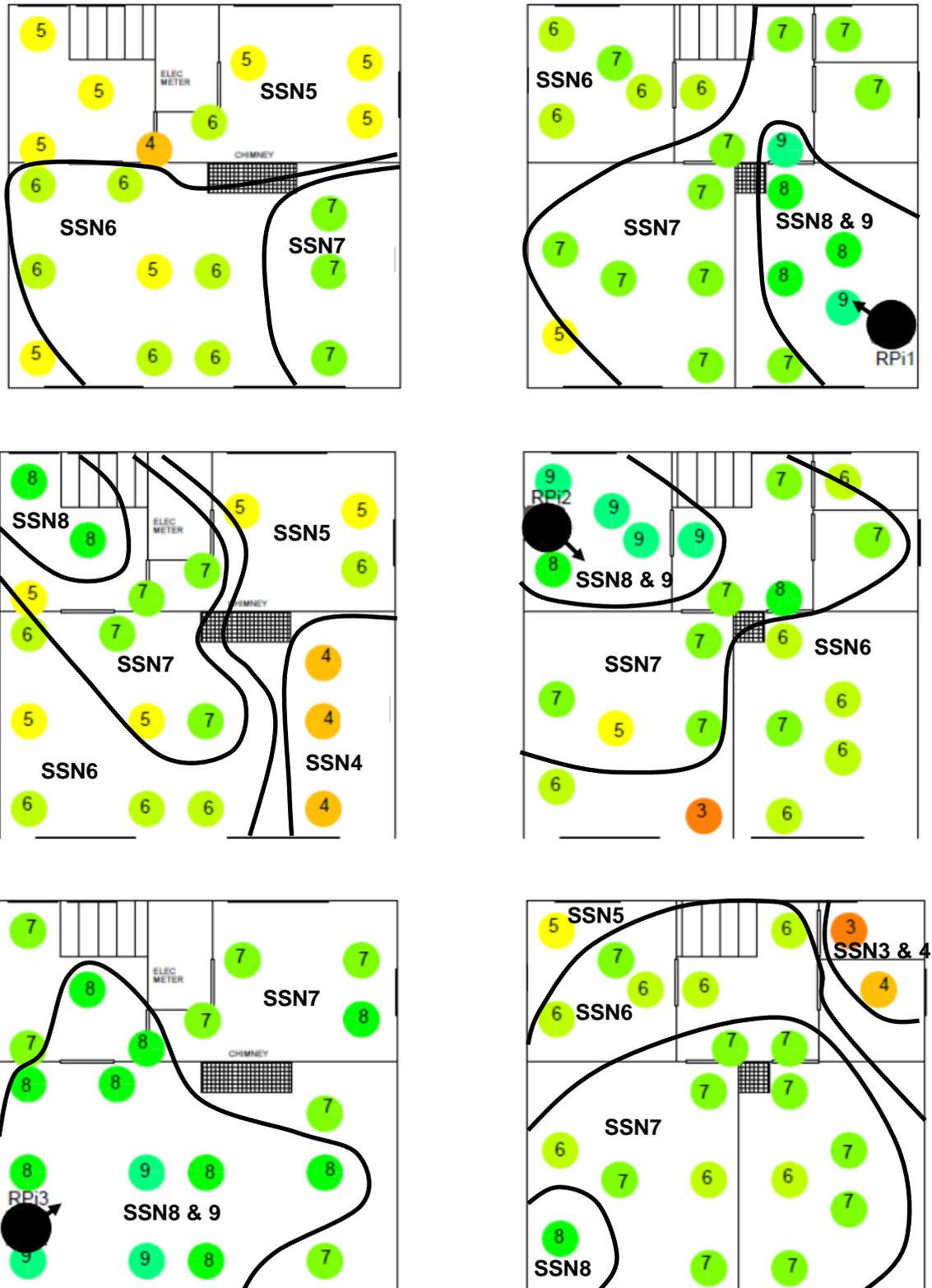
Figure 6.4 The signal strength contour maps of the prototype
