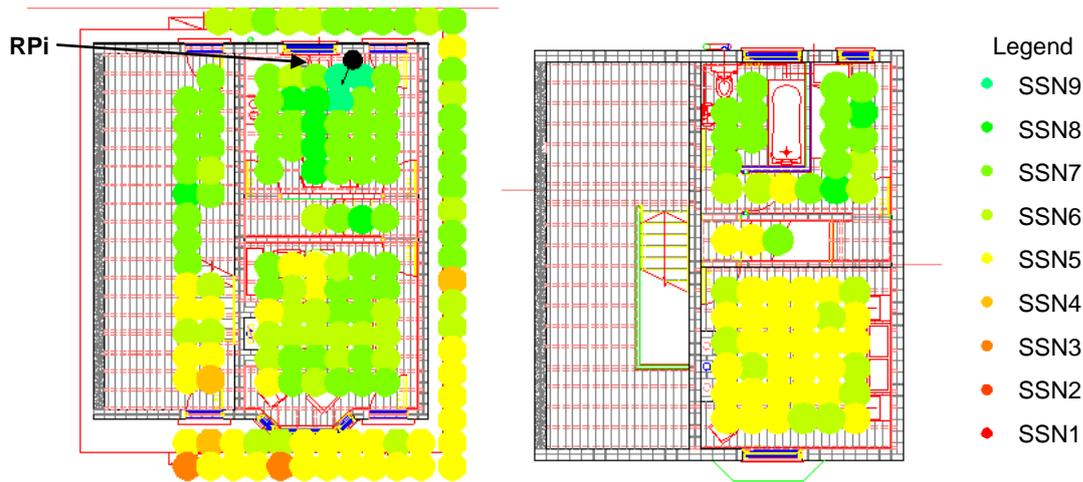
**Figure 4.16. Example of a heatmap from a test at the Salford Energy House (ground floor (left) and first floor (right)). The RPi position and reader direction indicated as in the kitchen and towards the opposite corner of the house.**
