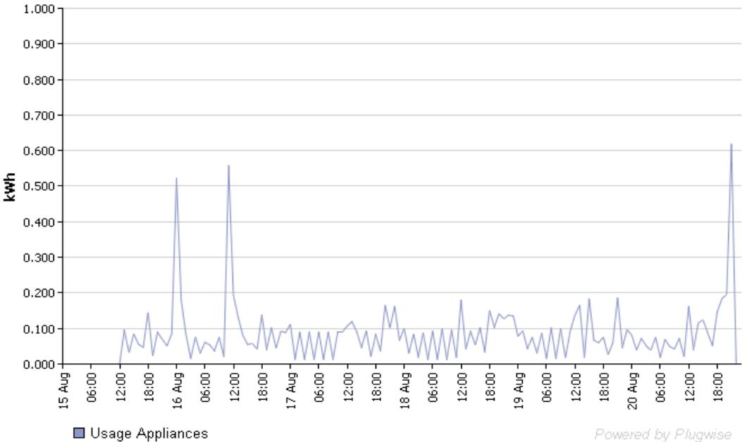
**Example of a graph showing total energy consumption for the network**
