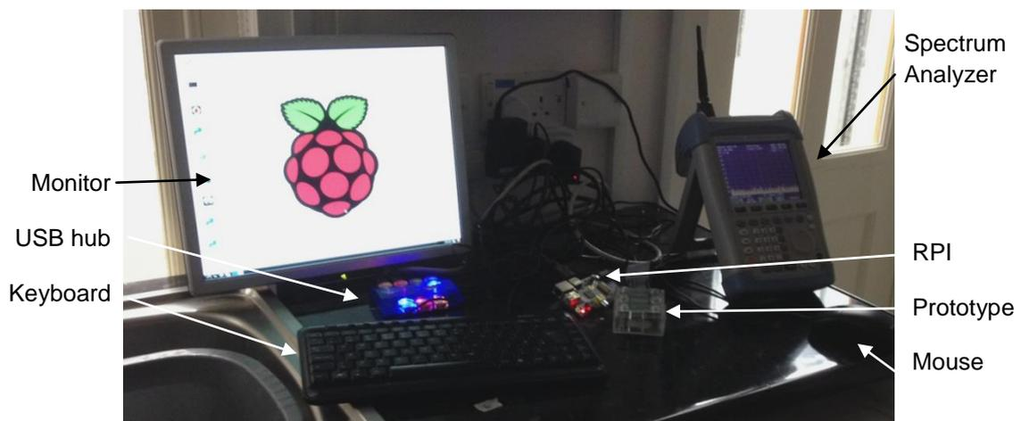
**Figure 4.1 Experimental Set-up with Spectrum Analyzer (from l-r monitor, keyboard, powered USB hub, RPi, prototype, spectrum analyzer, mouse)**
