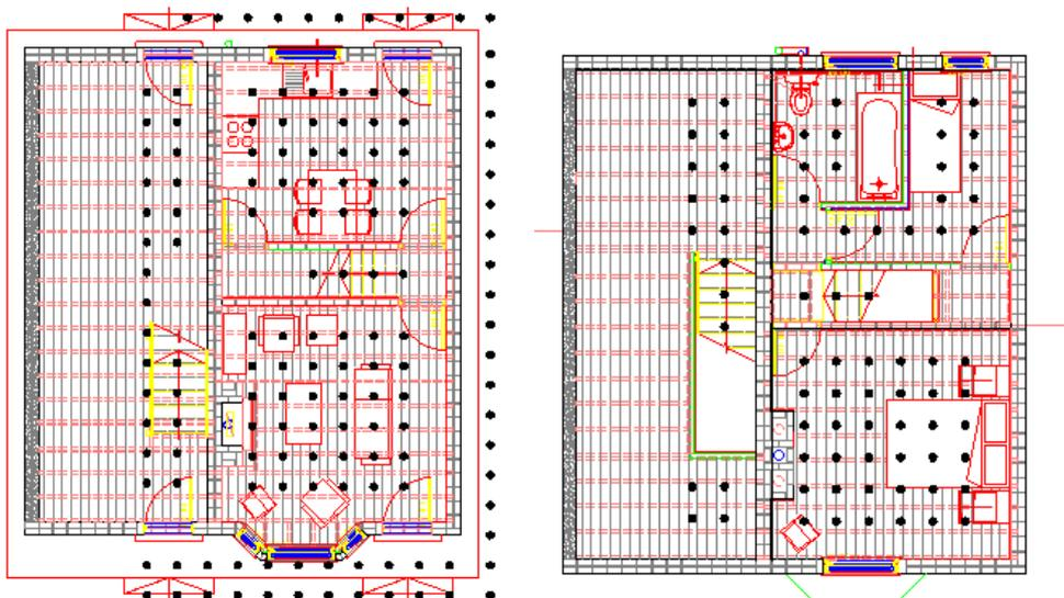
**Figure 4.4 The 222 sampling points at the Salford Energy House ground floor (left) and first floor (right)**
