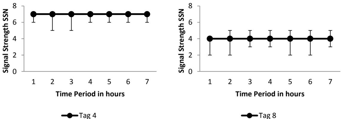
**Figure 5.46. Tag4 and Tag8 signal strength behaviour at the same location during Environmental Effects Test 2**
