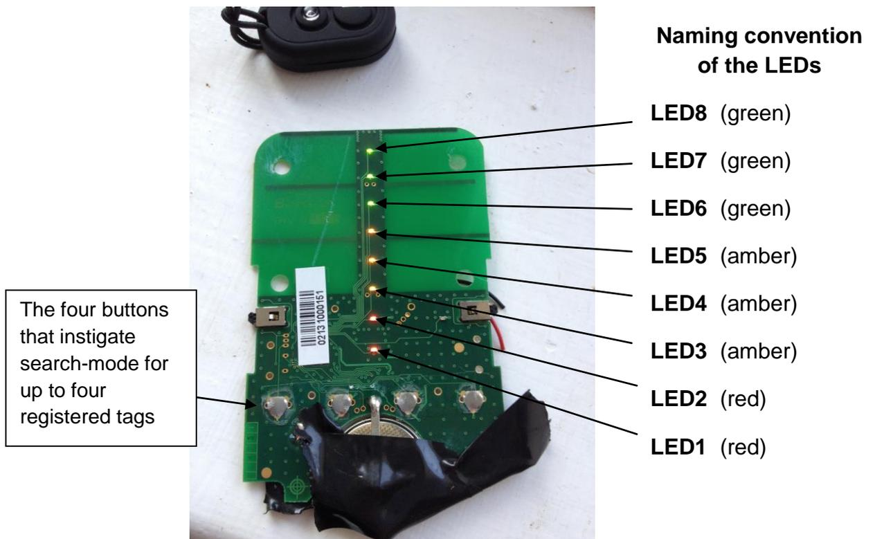
**The naming convention of the LEDs on the handheld unit PCB.**
