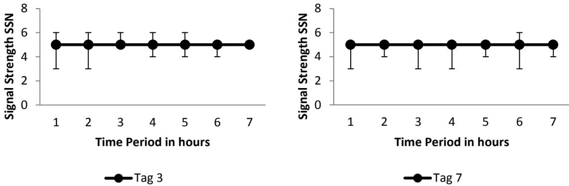
**Figure 5.45. Tag 3 and Tag 7 signal strength behaviour at the same location during Environmental Effects Test 2**
