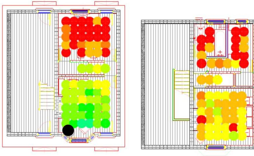
**Figure 5.1. Spectrum analyzer results from Test 1 at the Salford Energy House, ground floor (left) and first floor (right)**
