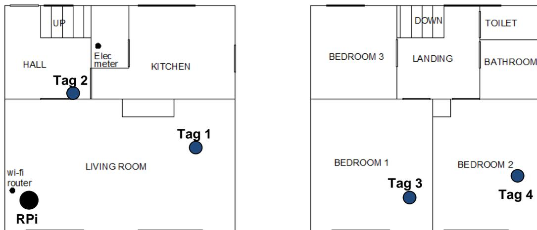
**Figure 5.28. Plan of Home1 ground floor (left) and first floor (right) showing the location of the RPi and four tags.**
