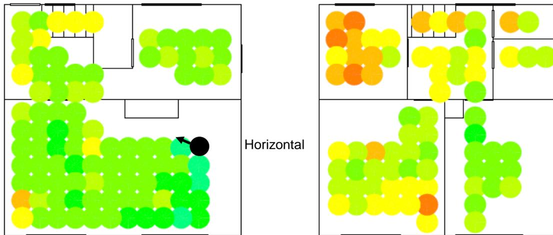
**Figure 5.20 Home1 Test 4 with the RPi placed in the living room, horizontal and directed towards the front door. Ground floor (left) and first floor (right)**
