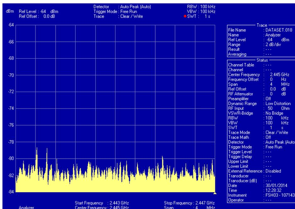
**Figure 5.6 Example of Spectrum Analyzer with no distinguishable signal strength visible above the background**
