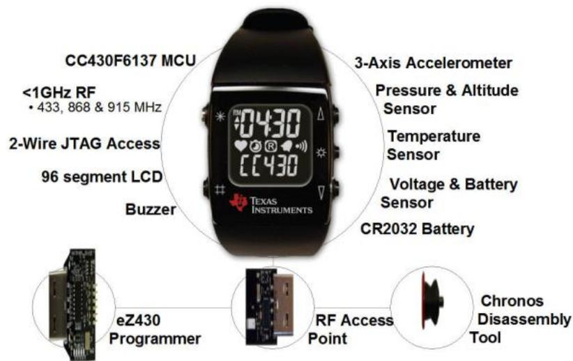
**Figure 3.2 The Texas Instruments eZ430-Chronos Development Tool (image from Texas Instruments)**
