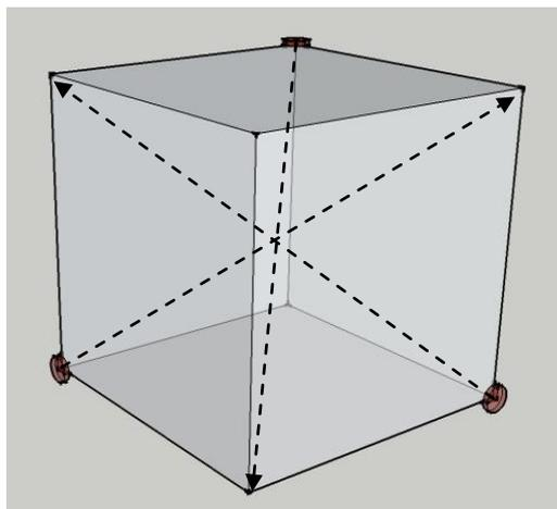
**Figure 4.9 The ideal locations for readers when using triple points to locate tags within the cube.**
