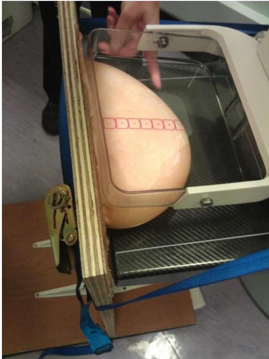
Figure 11.17 A compressed breast phantom during mammography
