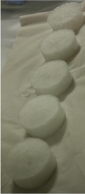
Figure 10.10 PVAL phantoms with 1-5 FTC
