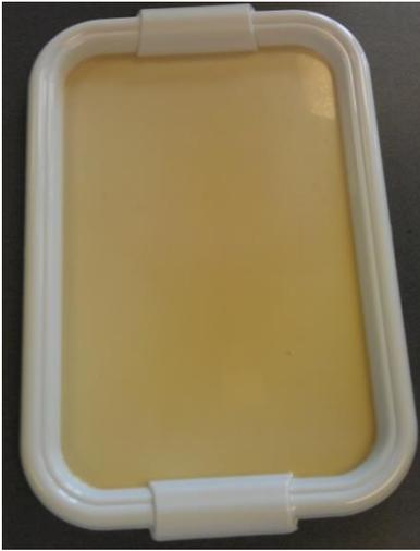
Figure 11.3 Top surface (chest part) of the breast phantom made up of latex paint.
