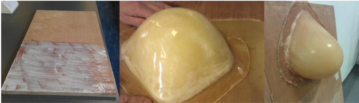
Figure 11.4 Attachment of the breast phantom/skin to the wooden torso
