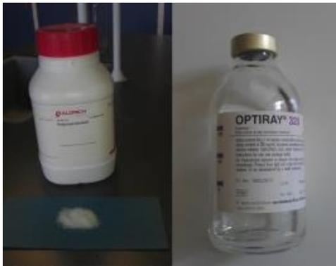
Figure 10.2 Left to right: PVAL from Sigma-Aldrich and Optiray 320 contrast agent.
