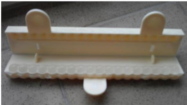
Figure 11.12 A plastic bead cutter to make round cancer mimicking lesions.
