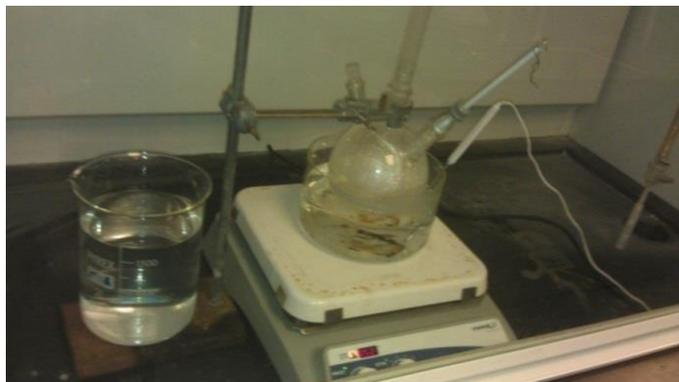
Figure 10.1 Equipment used inside a fume cupboard: A magnetic hotplate/stirrer, water bath, glass thermometer, digital thermometer, air condenser, and clamp stand.
