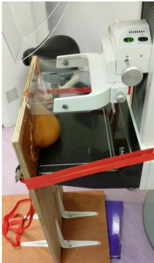
Figure 11.29 Mammography of a breast phantom attached to a wooden torso
