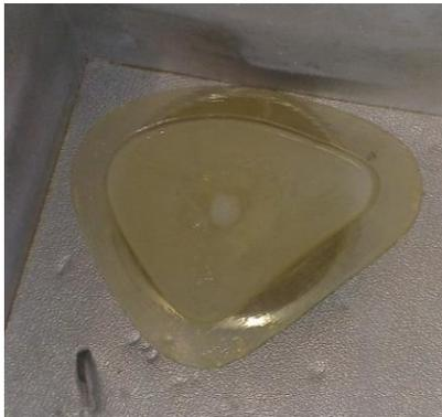
Figure 11.2 Breast phantom with an embedded lesion inside a breast mould painted with layers of latex paint.
