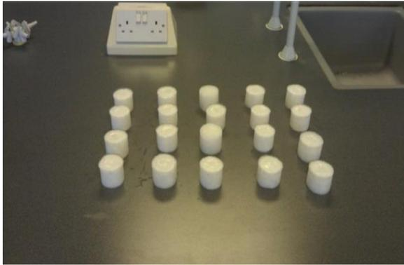
Figure 10.15 PVAL lesions, 2 to 6 FTCs, 4 phantoms per FTC
