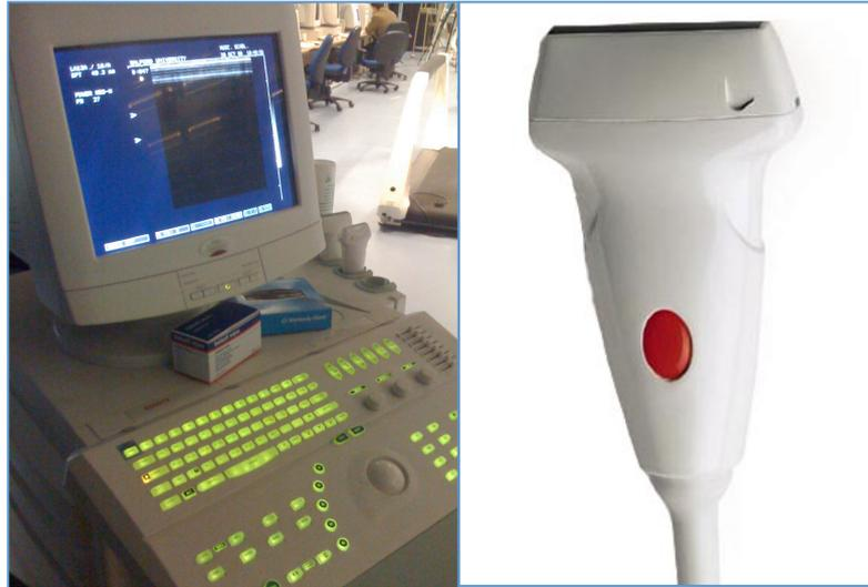
**Figure 3.4:** An example of a B-Mode ultrasound system and a 40mm probe transducer.
