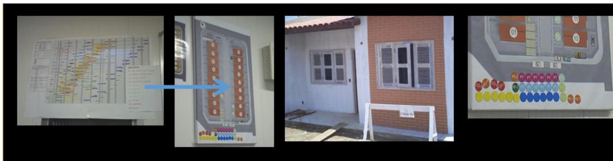
**Figure 26-Transforming construction schedules into more visual forms**
