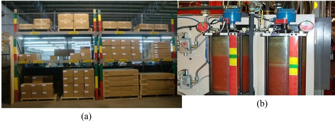
**Figure 13-Colour-coded inventory control in a warehouse (a) and material control on a machinery (b)**
