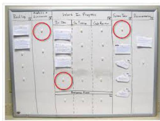
Figure 24-A process (workload) *kanban* example
