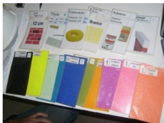
**Figure 16-Withdrawal *kanbans* in construction**
