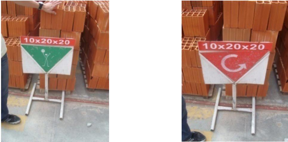
Figure 17-Pull-replenishment/production *kanbans* for bricks
