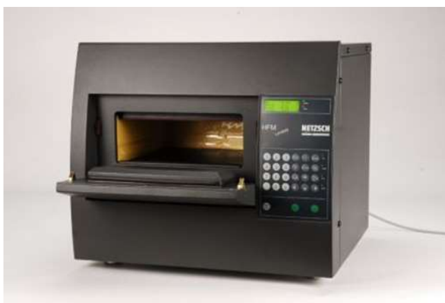
Figure 3: FOX 600 heat flow meter in the thermal lab
