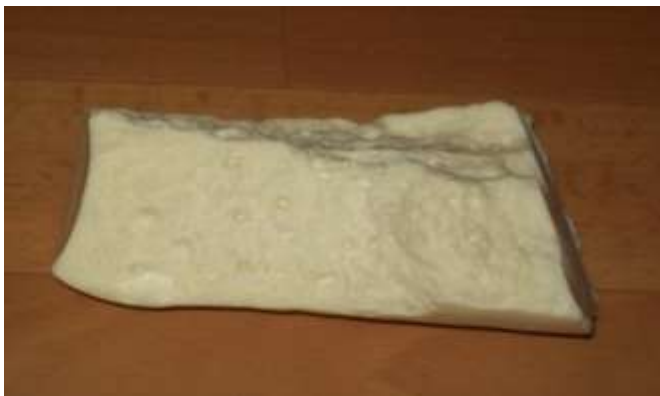
Figure 6: aerated soap created by the vacuum method
