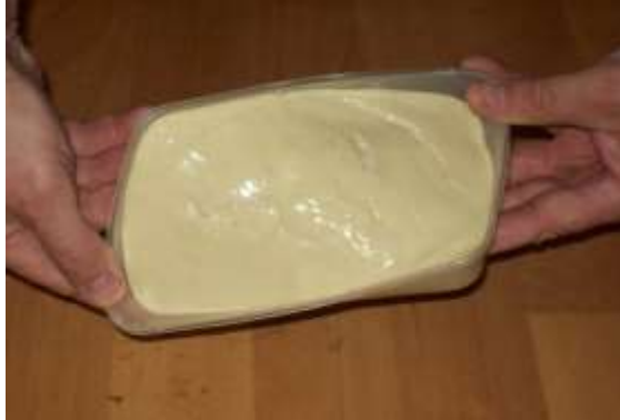
Figure 4a: This waste engine oil soap remained in a “blancmange” state
