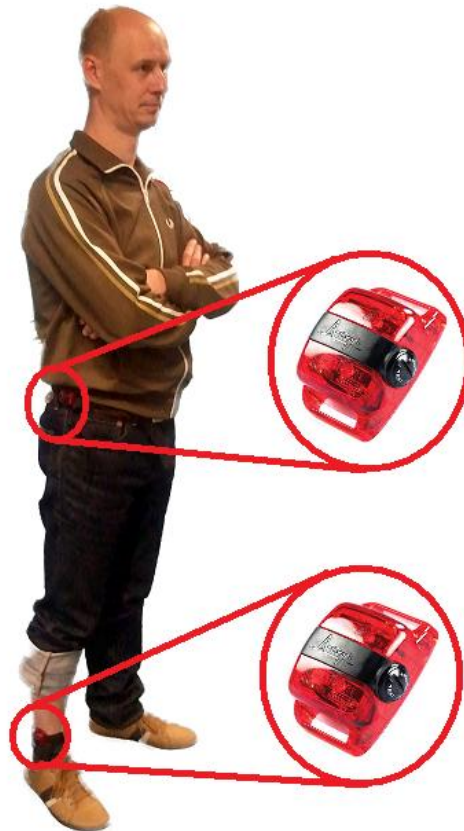
Figure 10: Accelerometer placement at the ankle and at the waist above the hip.
