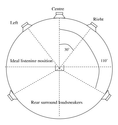
Figure 2: Loudspeaker Setup for 5.1 Surround Sound
