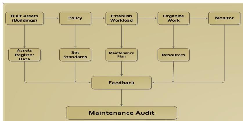
**Figure 2.2: Built Assets Maintenance Management Model/Framework** (Adapted from Allen, 1993)
