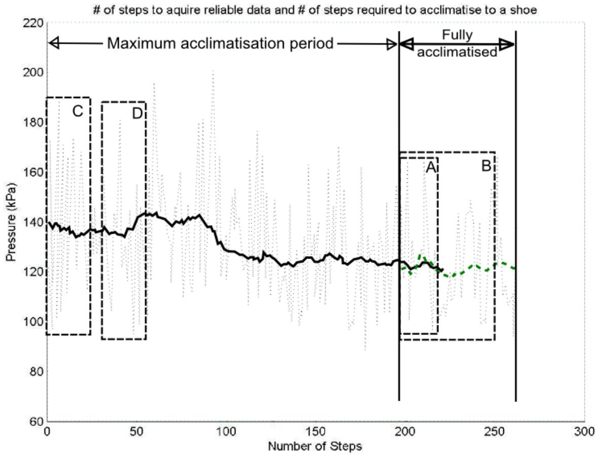
Figure 40: A depiction of the algorithms used to calculate the acclimatisation period and the number of steps required to produce an average representative step.
