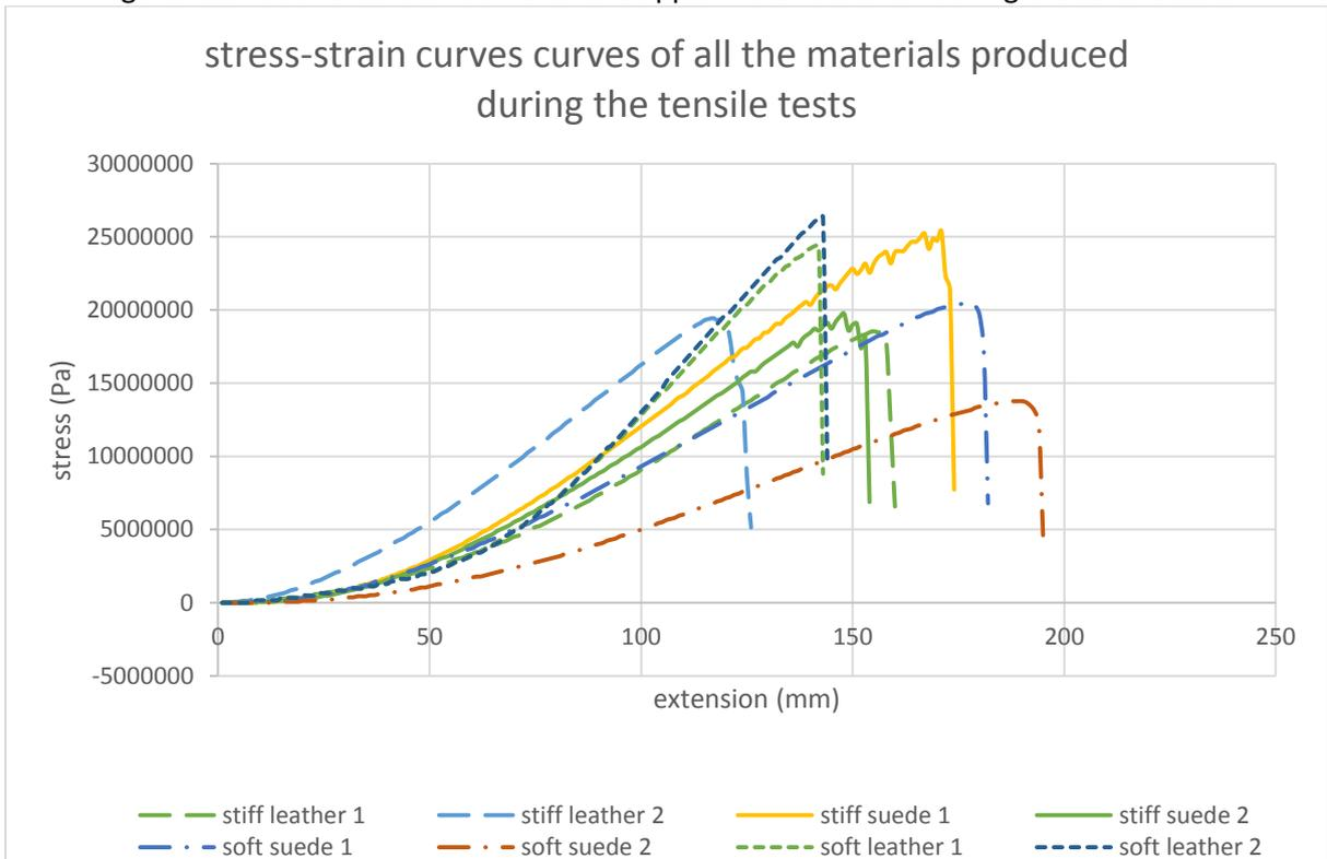
Figure 140: stress-extension curves for upper materials taken during the tensile tests
