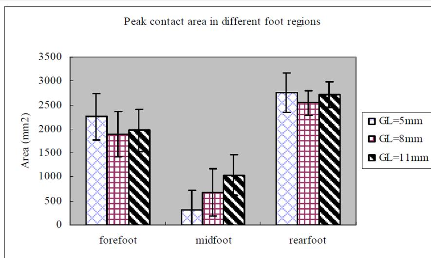
Figure 12: The peak contact area for a range of foot regions, using varied shank curves. GL represents the distance from the waist of the last to the line joining the heel breast to the ball tread. Taken from Cong et al [28]
