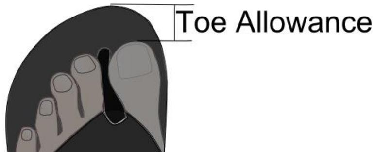
Figure 24: Toe allowance of a shoe
