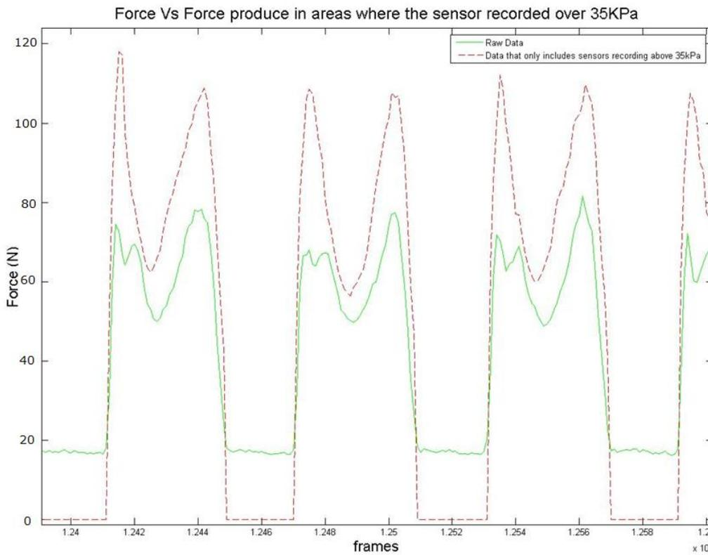
Figure 36: A comparison between raw and filtered force data, zoomed in to three random steps
