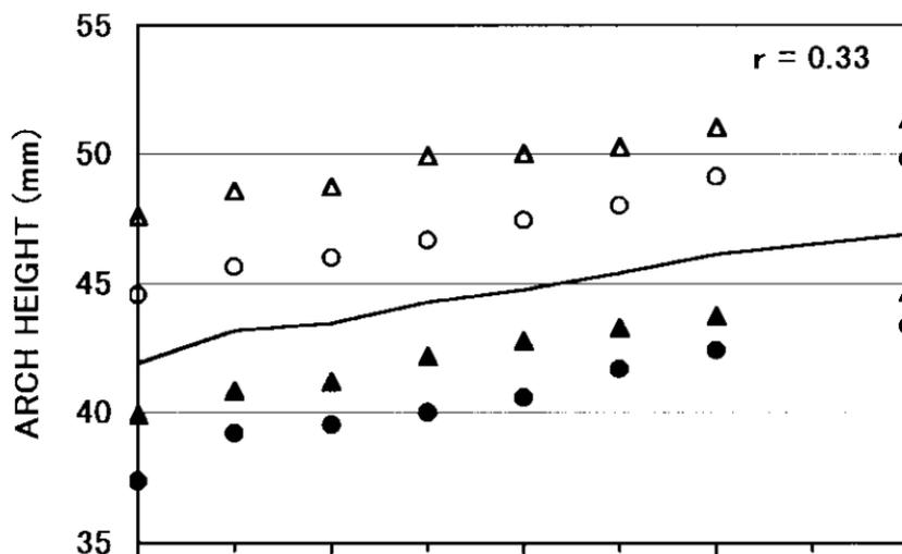
Figure 29: The effect of heel height on longitudinal arch height [97] with heel heights of 0, 5, 10, 15, 20, 25, 39, and 40 mm. Filled shapes represent low arched subjects, empty shapes represent high arched subjects, triangles represent subjects with weak rearfoot pronation, circles represent subjects with strong rearfoot pronation, and the line shows the overall mean values.
