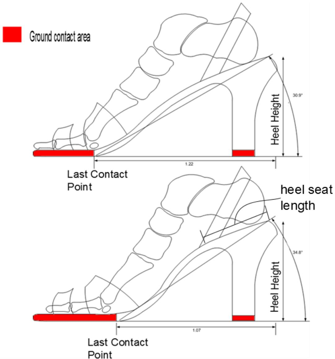
Figure 3: The effects of last contact point location, when heel height is fixed. The red areas show the regions of the shoe which are in contact with the ground. Horizontal measurement shows the last contact point distance and the angle shows the projection angle from the apex of shoe to highest point
