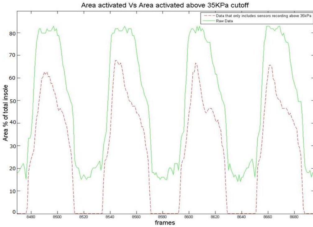
Figure 35: A comparison between raw and filtered area data, for four steps
