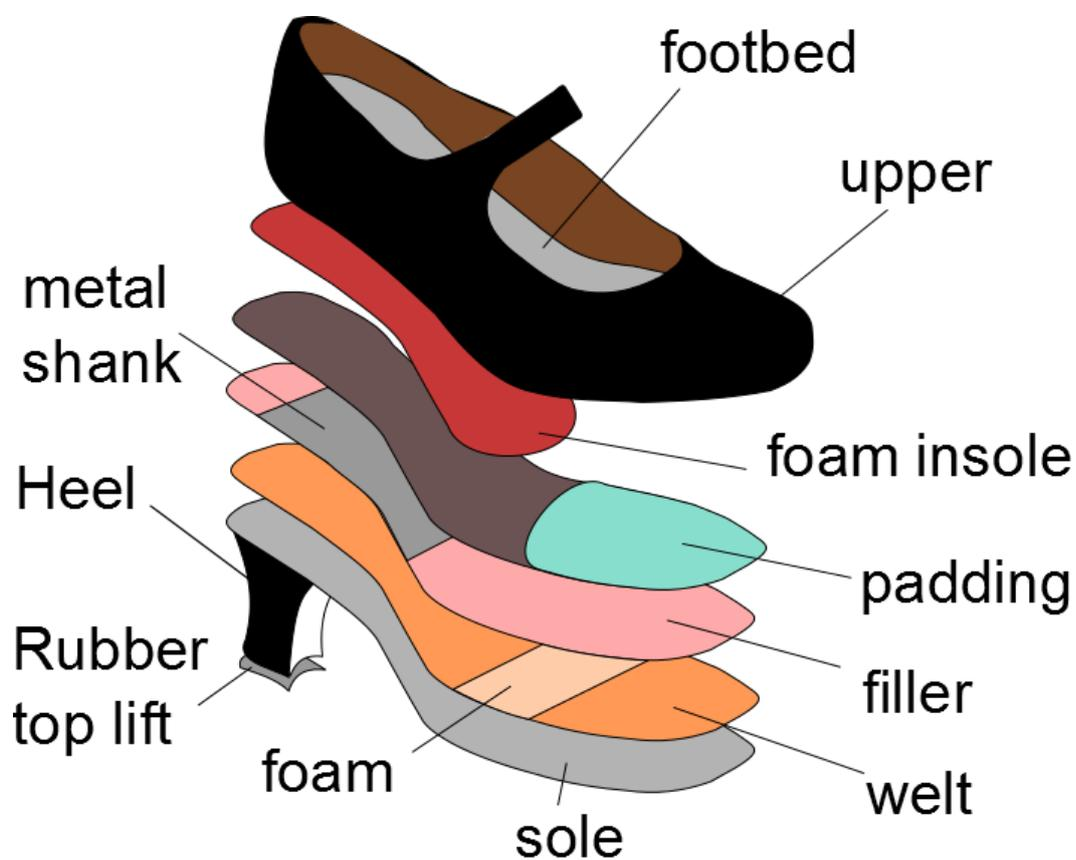
Figure 2: The structure of a high heeled shoe
