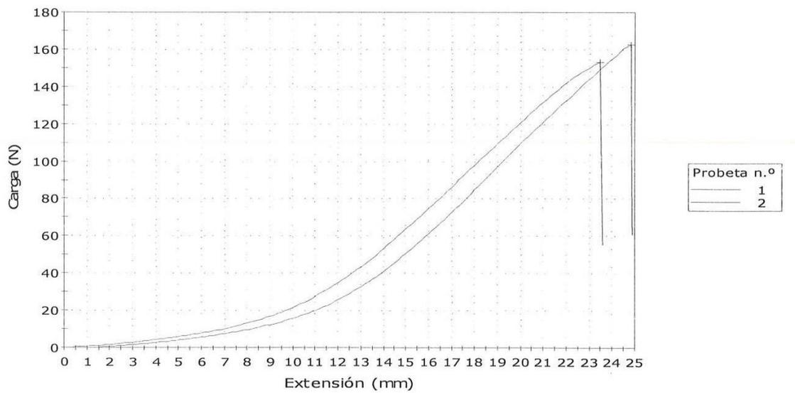
Figure 138: Plot provided by INESCOP showing the force against extension curves for two materials.
