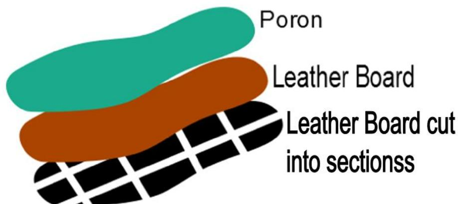
Figure 91: layers of the insoles
