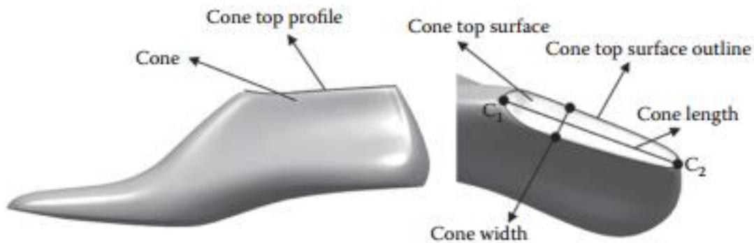
Figure 8: cone of the shoe-last [38]
