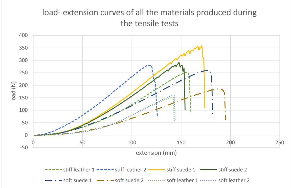
Figure 139: load- extension curve for the upper materials taken during the tensile tests
