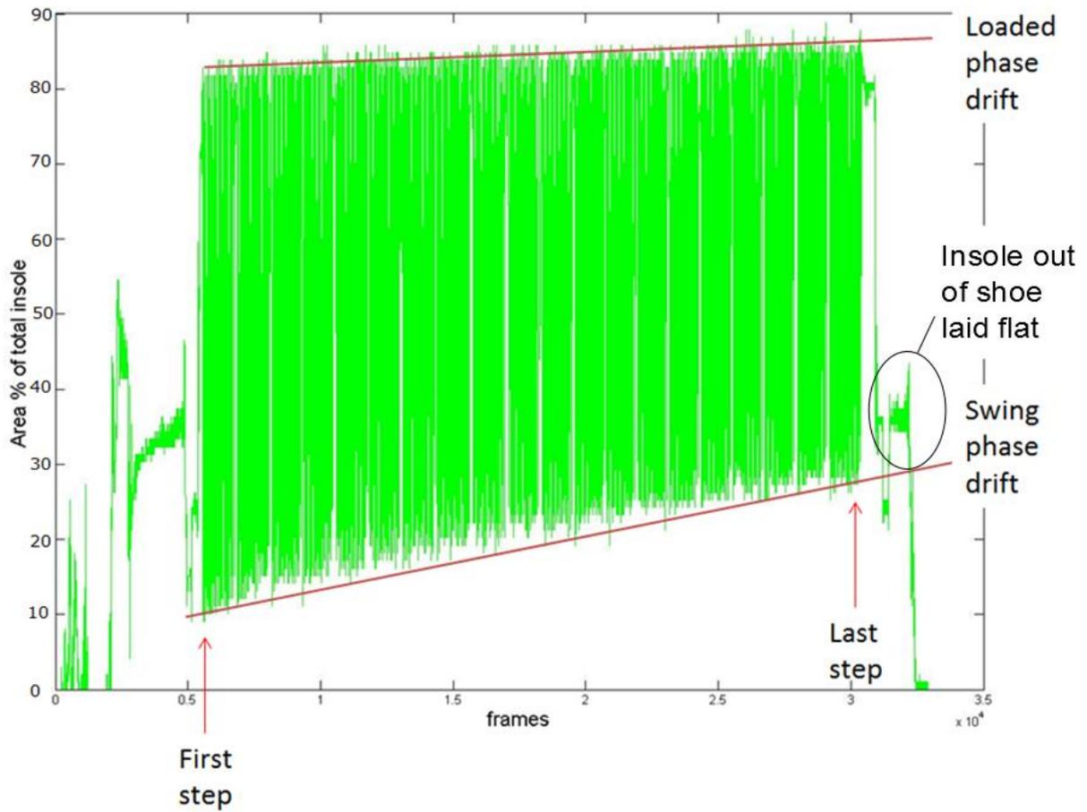
Figure 33: Drift in the raw area data
