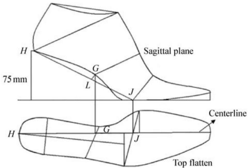
Figure 11: diagram showing the definition of GL taken from Cong et al 2011 [78]
