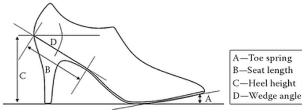
Figure 16: Footbed parameters [38]
