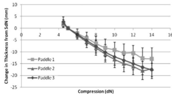
**Figure 2** Paddle comparison—mediolateral oblique view. Paddle 1, small (15×29 cm); Paddle 2, medium (18×24 cm); Paddle 3, large (24×30 cm).
