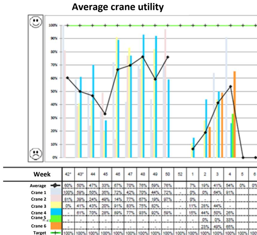
Figure E.14: Overall crane utility, Plant E
