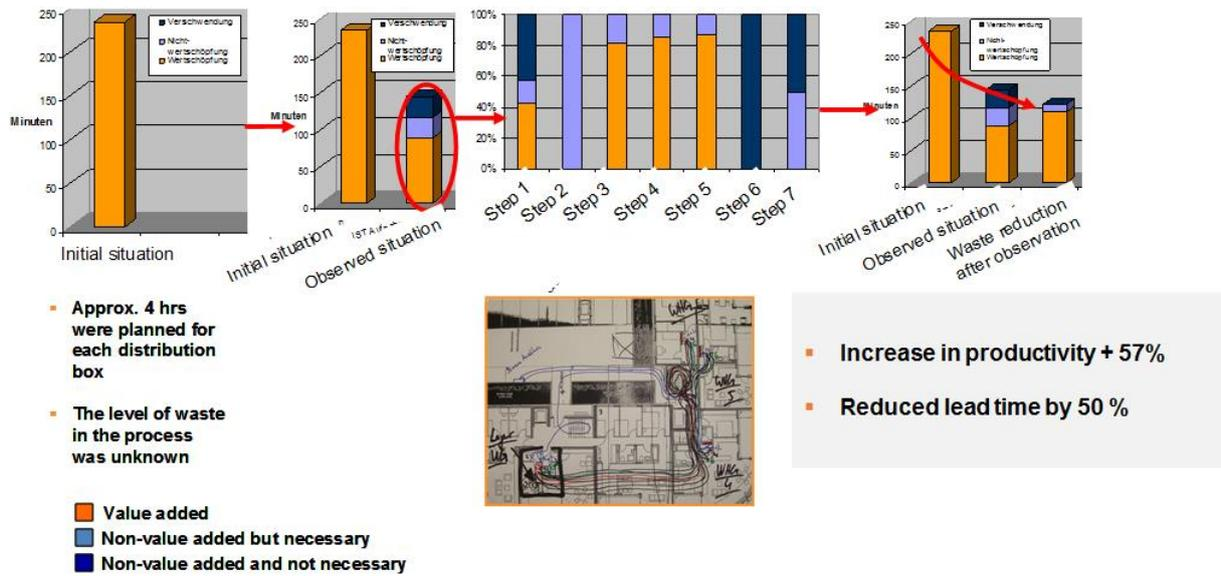
Figure C.1: Observation of the electrical assembly process
