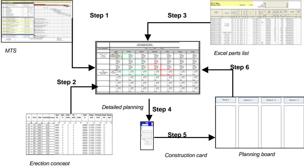
Figure 7.30: The additional pre-planning steps as part of the LCM models adaptation to power plant construction.
