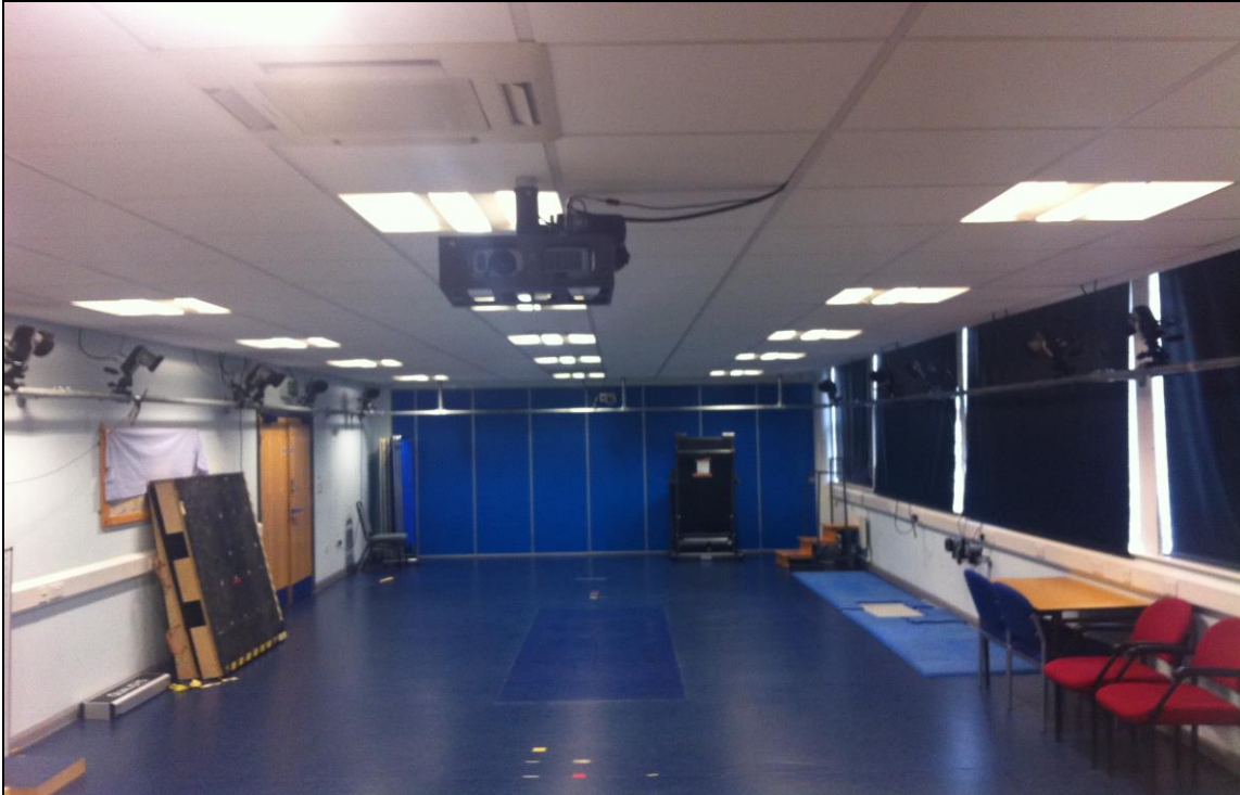
Figure 3-3: The sixteen-camera Qualisys Oqus motion analysis system and four force platforms (AMTI BP400X600, AMTI, USA) at gait lab.
