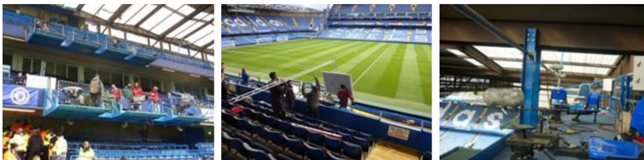
Figure 3 - Chelsea test shoot: camera platform (left), calibration of the OmniCam (middle), Soundfield® mics and stereo pair (right)
