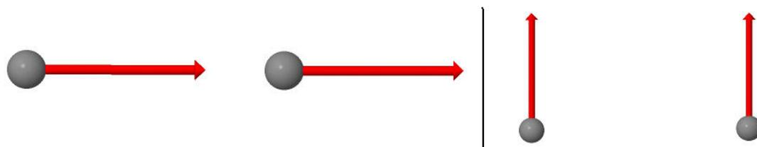
Figure 5-32: (Left) LA mode of vibration of frequency  $154 \text{ cm}^{-1}$ ; (Right) TA mode of vibration of frequency  $47 \text{ cm}^{-1}$ .
