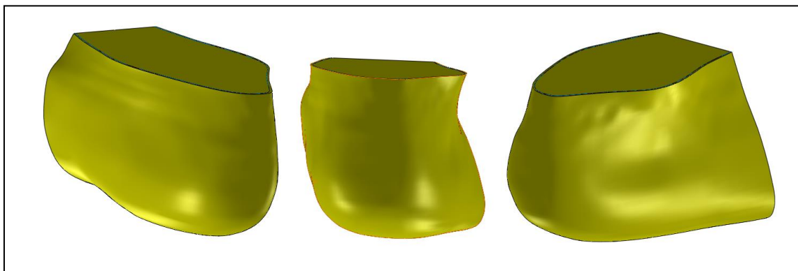
Figure 3.32: The 3D solid model of the heel region as a single layer structure.
