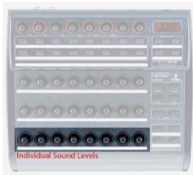
Figure 3 : Soundscape simulator controller, showing controls for sound source
