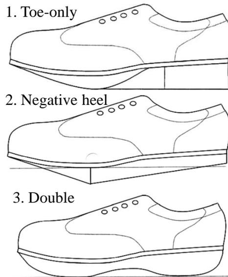
**Figure 2. 3: Three different rocker sole designs, 1) toe-only, 2) negative heel and, 3) double.**
