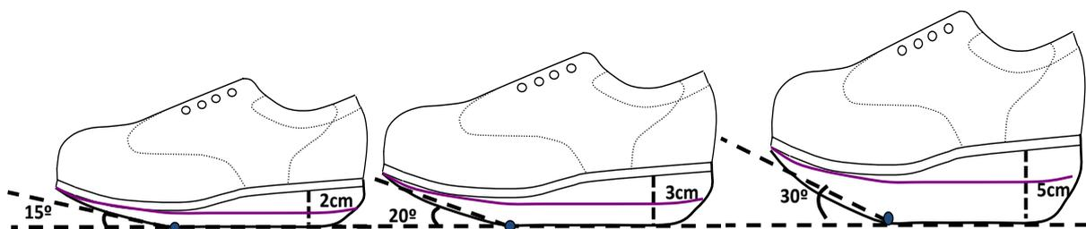
**Figure 3. 20: The increase in heel height caused by increasing the rocker angle.**
