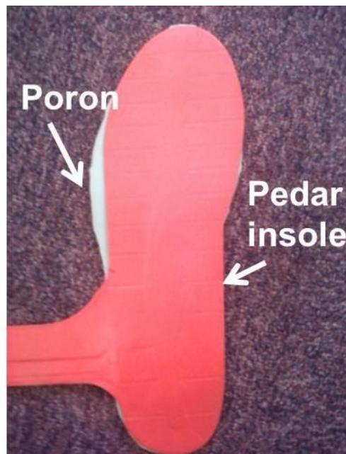
**Figure 4. 2: Pedar pressure sensitive insole attached to the top of the custom made poron insole.**
