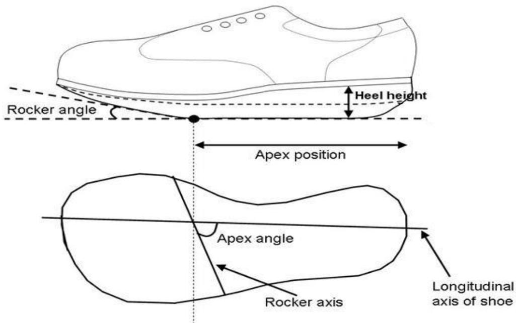
**Figure 3. 1: Definition of the rocker outsole design features (rocker angles, apex position and, apex angle).**
