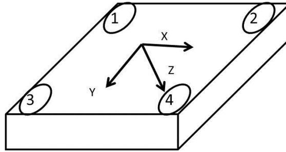
**Figure 5. 7: Piezoelectric force plate schematic.**
