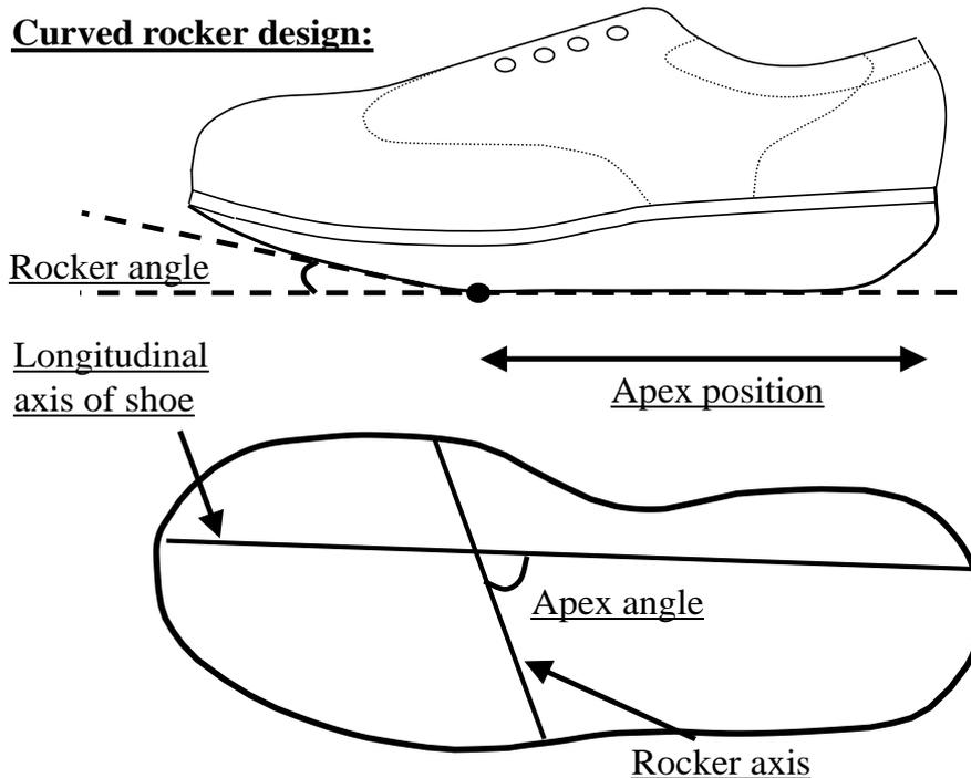
**Figure 2. 4: The traditional rocker design and the curved rocker design with the three design features: 1) rocker angle, 2) apex position and 3) apex angle.**
