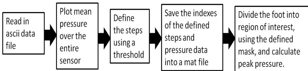
**Figure 3. 3: Flow chart representing the code used to process and analyse the pressure data.**
