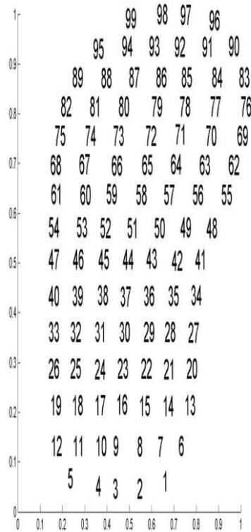
**Figure 3. 7: Left side Pedar insole. Sensor number shown on the plot and corresponding x and y co-ordinates are given by the axes.**
