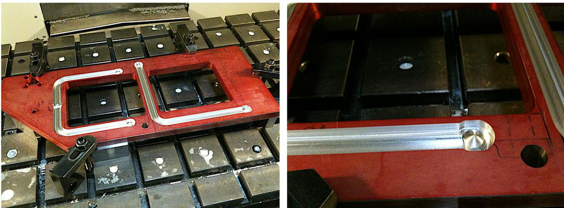
**Figure 4.5:** Second prototype consisted on a “C” and a “L” shape machined in *CNC* Vertical Machine centre using high- grade hardened aluminium in Minalum de México company.
