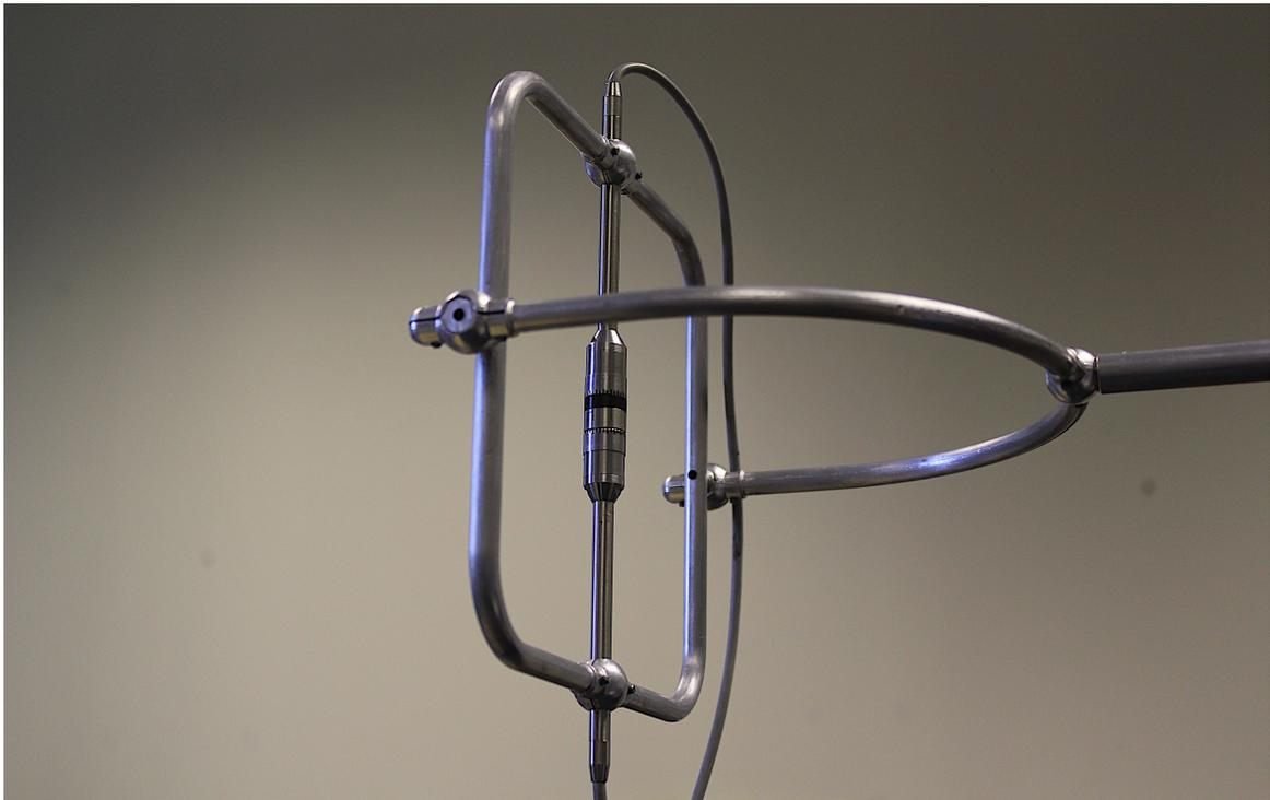
**Figure 4.9:** The third prototype of rotation cradle guaranteed the accuracy of the positioning of the face-to-face p-p probe configuration with the highest accuracy, the rotation of the p-p probe at 90 degrees.
