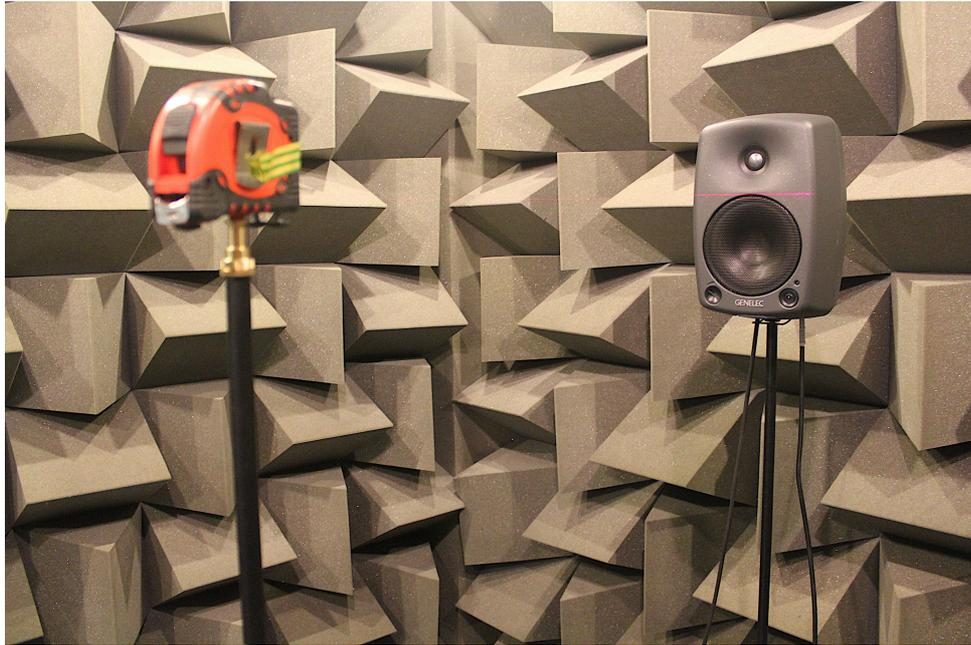
**Figure 5.1:** Acoustic centre of the near field monitor *Genelec* 8030A used in the measurements located by the laser pointer located at tangent to the woofer at a height of 19 cm from the Iso-Pod™ table stand of the monitor and valid from a distance larger than 0.7 m (2007).
