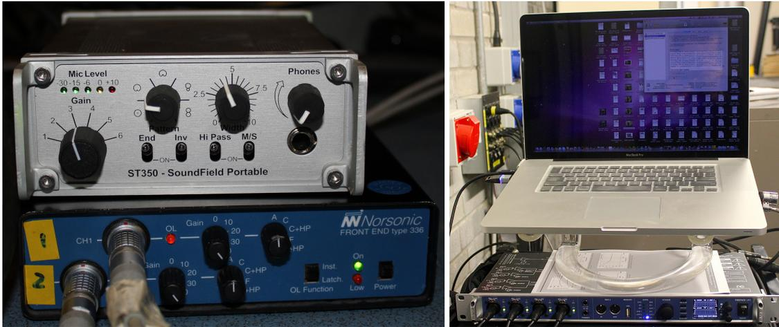
**Figure 5.7:** The equipment used for the last measurements. The photo of the left side shows the preamp for the *Soundfield* microphone ST350 and the Norsonic signal conditioner type 336 for the one-dimensional p-p probe. The photo of the right shows the *RME Fireface UFX* sound card which uses digital preamps connected to a *DAW Pro Tools 9* running over a *MacBook Pro*.
