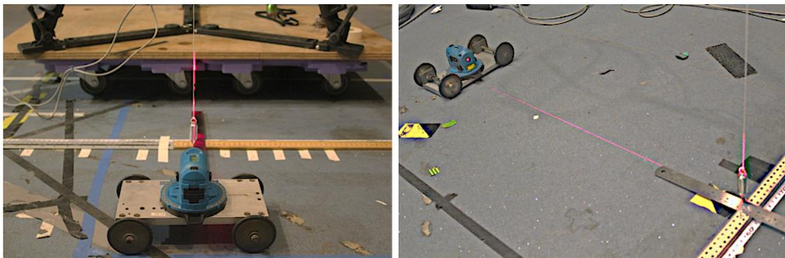
**Figure 5.5:** The laser pointer controlled in a railway trolley cart and the perpendicular steel ruler serving as a guide with the plum bob pointing at the ruler.
