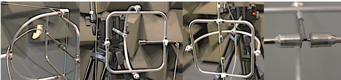
**Figure 5.11:** Different configurations of spacers tested on the p-p probe.
