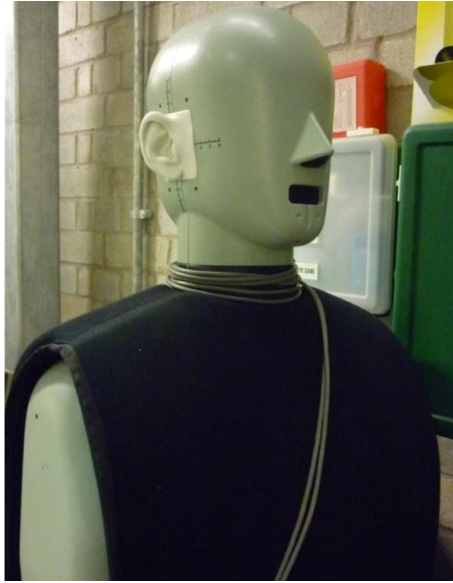
Fig. 2.8 Brüel & Kjær HATS dummy head used for binaural recording
