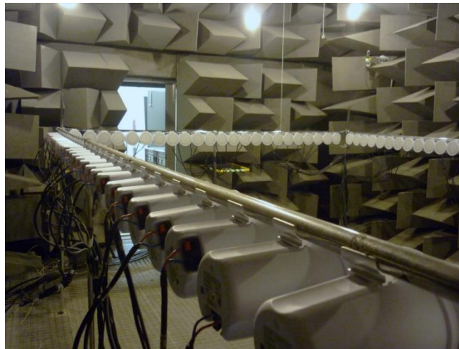
Fig. 3.26 Semi-portable WFS installed in the anechoic chamber
