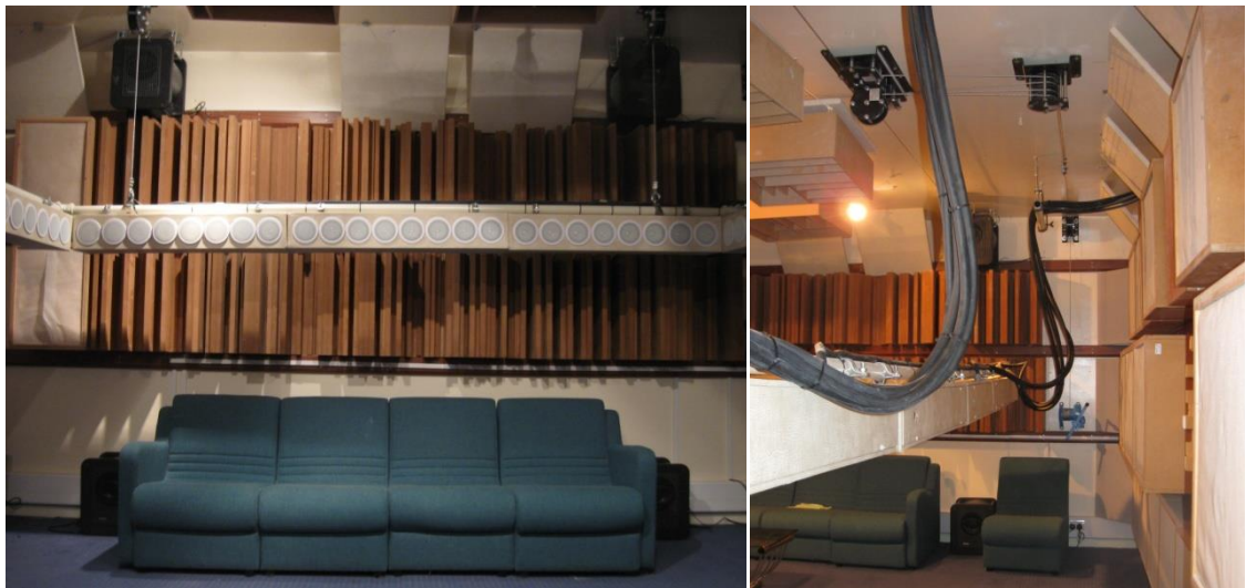
Fig. 3.28 Loudspeakers suspended on winch system in listening room
