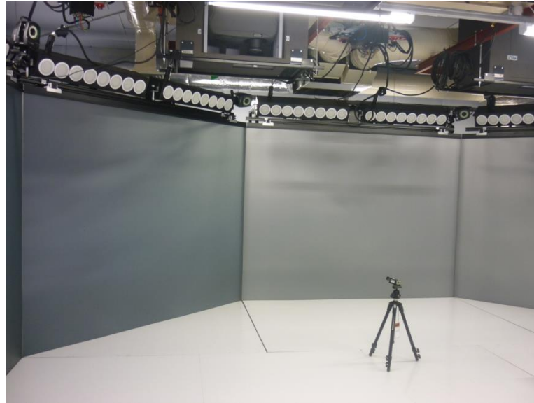
Fig. 3.30 128 channel WFS system installed in the Octave virtual reality lab at the University of Salford
