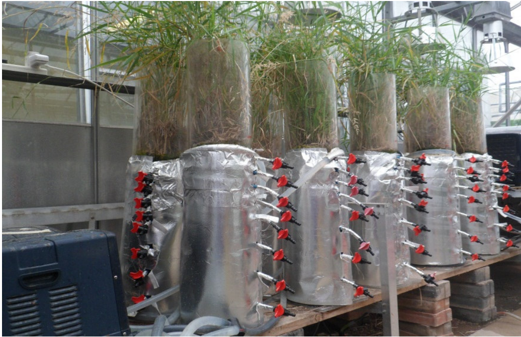
Figure1: Laboratory set-up of the vertical-flow constructed wetland system located within a greenhouse on top of the roof of Newton Building of University of Salford, UK
