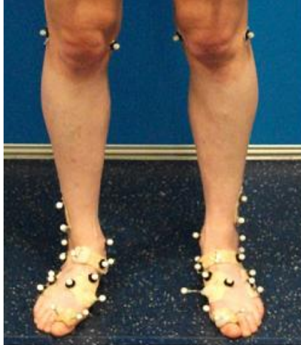
Figure 5.7- Anterior view of the placement of the Salford foot model plates and all anatomical markers on the foot and leg
