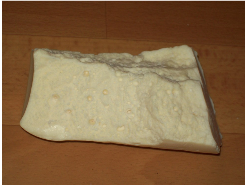
Fig. 5: aerated soap created by the vacuum method. (Read, 2012)
