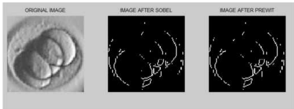
Figure 4.4 Image after applying Sobel and Prewitt
