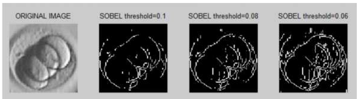
Figure 4.5 Using different thresholds on Sobel
