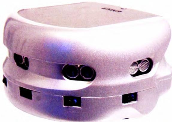
Figure 6.15: Khepera III mobile robot.
