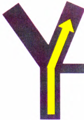
Figure 6.1: Example for decision support in car navigation systems - Car navigation systems very often provide an additional graphical representation of junctions to support the driver in choosing the correct road (own depiction)
