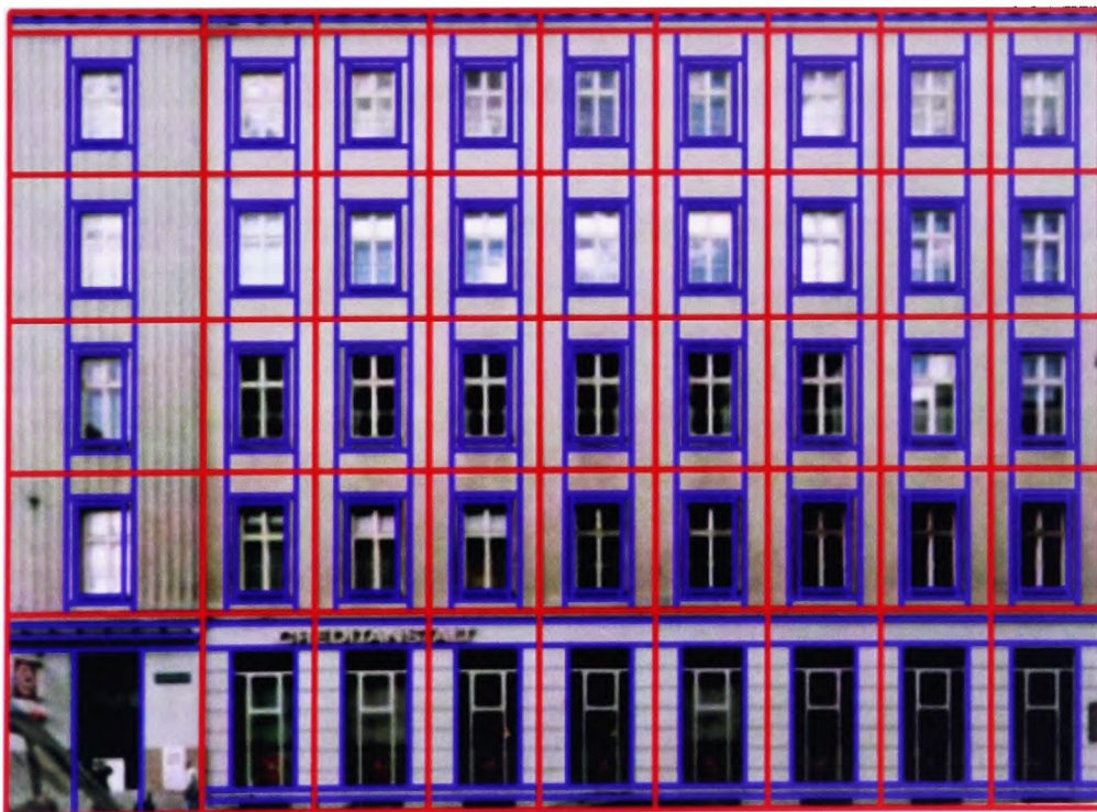
Figure 2.5: Façade grammars - Façade that is subdivided into smaller elements. A grammar is derived from this description(from Müller et al. (2007))
