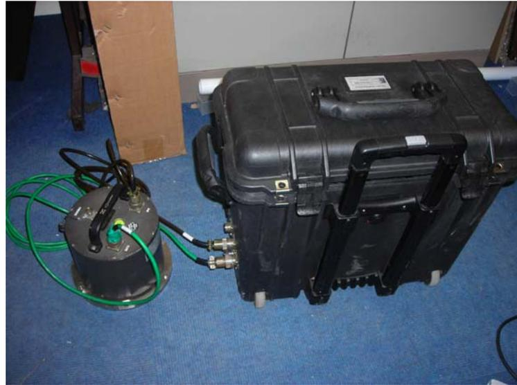
**Figure 1** Guralp CMG-5TD force-feedback strong-motion accelerometer
