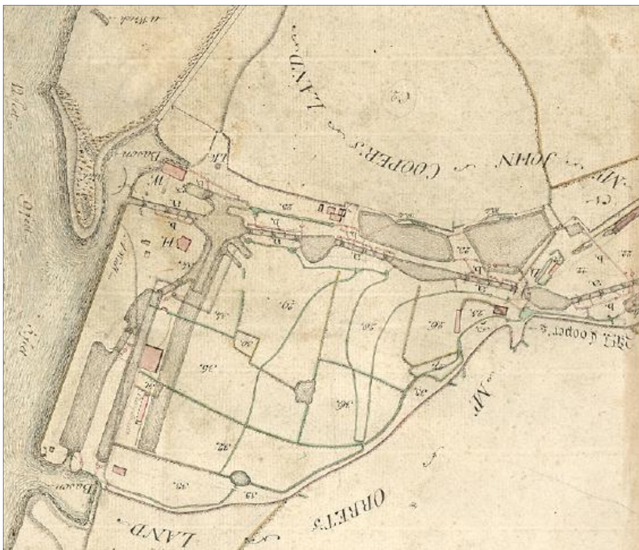
Fig 10.14: The Runcorn terminus in 1785 according to Foulkes' survey, showing the line of the old locks with its tidal lock to the River Mersey and the original dry dock to the north. This map has been annotated to show the addition of the old tidal basin to the south-west. To the right of this is the middle or coal basin, and east of that is the old basin. Since the line of the new locks are not shown these additions much pre-dated the mid-1820s. (Courtesy of Salford City Archive, Bridgewater Collection).
