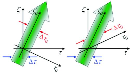
FIG. 1 (color online). Illustration of the relationship between pulse durations in the laboratory frame  $(\tau, \zeta)$  and the rest frame  $(\tau_0, \zeta_0)$ . The two distinct spatiotemporal regimes are: (a)  $\text{sgn}(s\kappa) = +1$ ; and (b)  $\text{sgn}(s\kappa) = -1$ .
