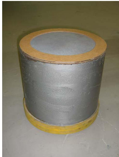
B: Clamped membrane on large sample holder
