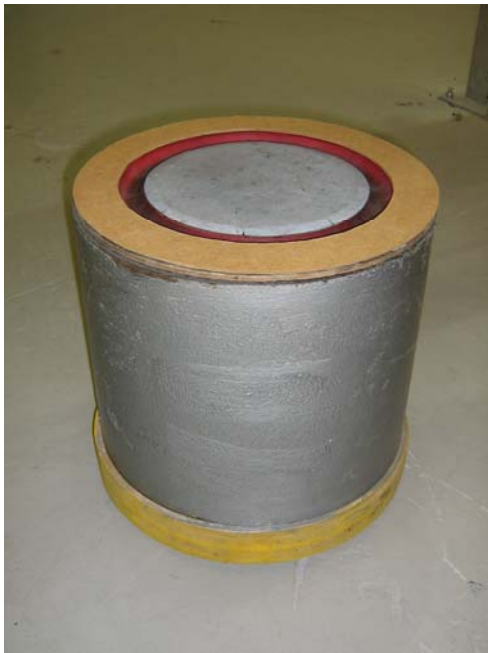
A: Surround mounted membrane on Large sample holder
