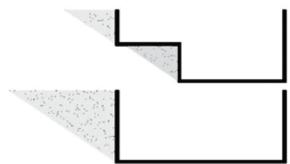
Figure 15: Effect of plan on self-shadowing
