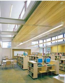
Figure 6: (Left) The classroom and activity area with large glazing; (Right) The library utilizes clerestory windows for diffuse daylighting (Ben Franklin Elementary School, Kirkland Washington, US – Confirmatory Case) (Source: Mahlum Photography)
