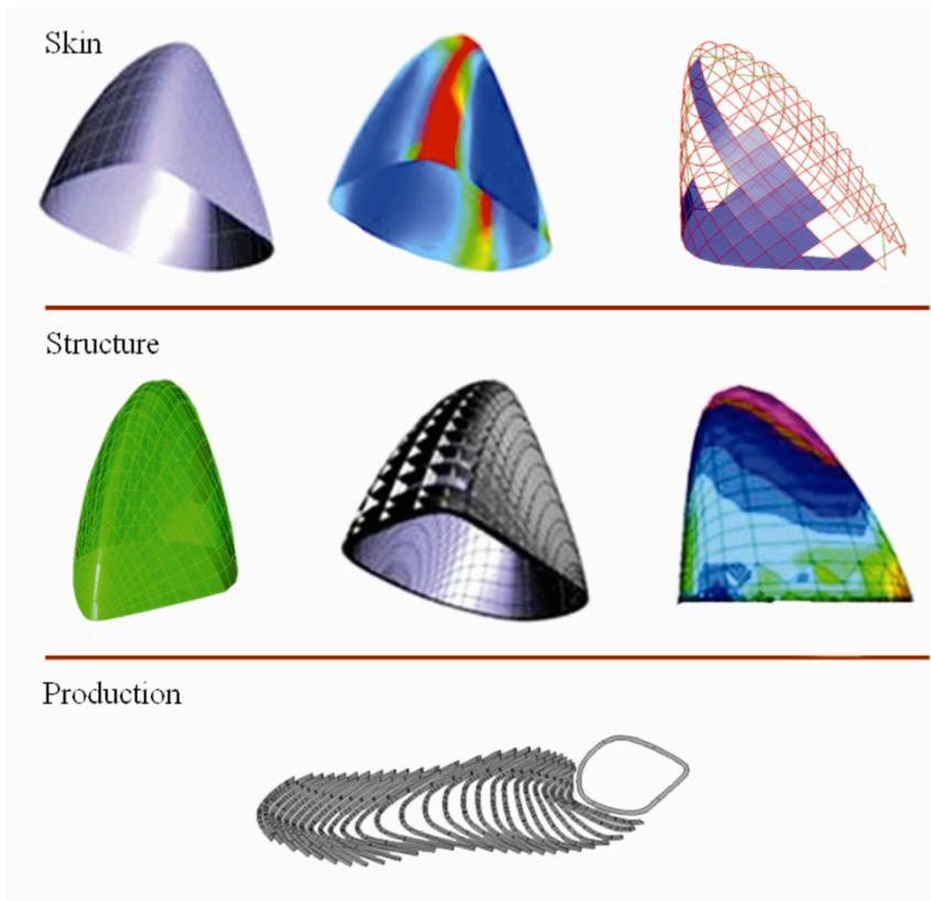
FIG 11: Compatible solutions selected for the cladding patterns, the structural configuration and the laser cut structural elements
