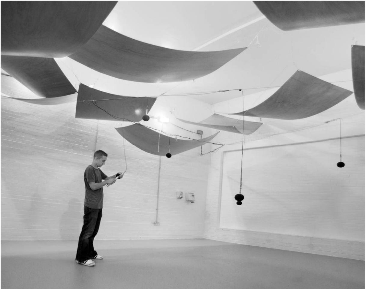
*Figure 1.6: Reverberation chamber with suspended scattering panels*
