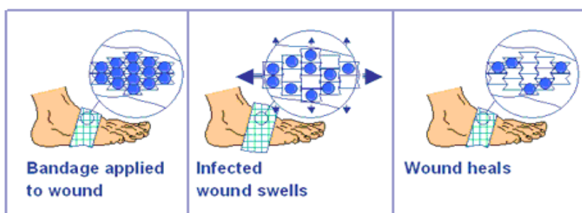
Fig 7: Structural changes of an Auxetic bandage Source: www.azom.com
