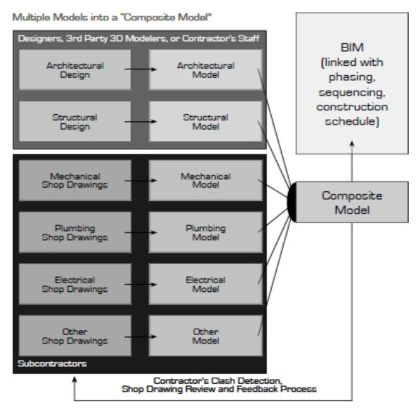
Figure 2 : Multiple Model in Implementing Building Information Modelling For a Single Project
