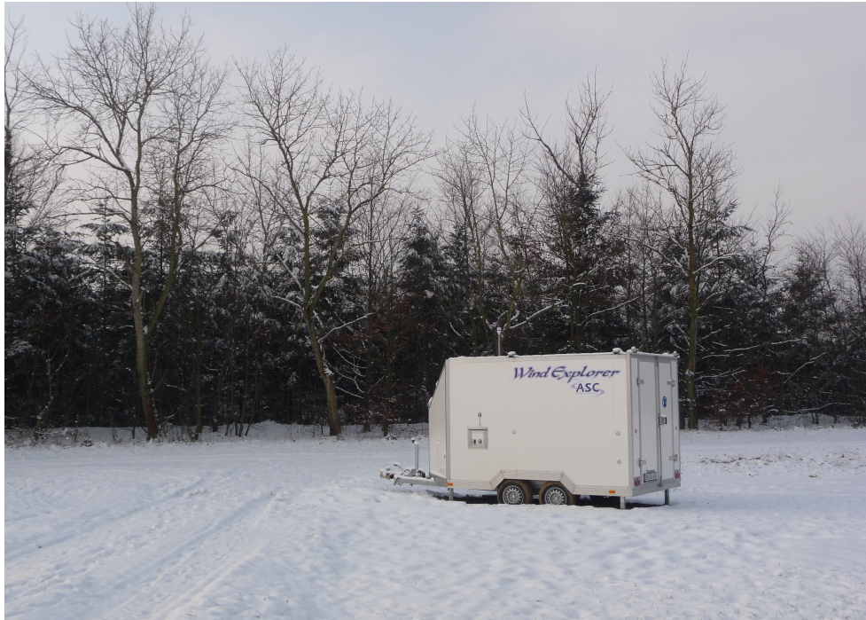
Figure 3.7.5 – ASC4000 Wind Explorer SODAR set-up at Wind Test Grevenbroich's turbine testing field in Germany.
